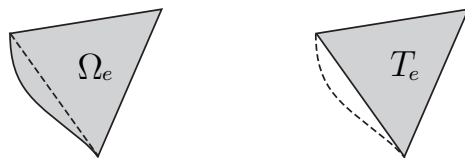
Figure 5: Actual element \Omega_e (left) and triangle T_e defined using its vertices (right) in the physical domain
