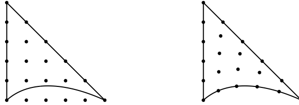
Figure 8: 5th-order nodal distributions in I_e : for equally-spaced nodes in the straight-side triangle (left) and adapted to the NURBS side (right)
