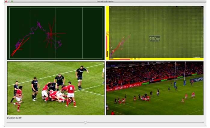
Fig. 8. Thumbnail viewer of NMV. The user can interact with the NMV by adjusting the duration slider to animate the motion path. The corresponding video keyframes are also displayed. The user can overlay additional information onto the video, including the NMV and distances between the team, the forwards and backs, in both the x and y directions.
