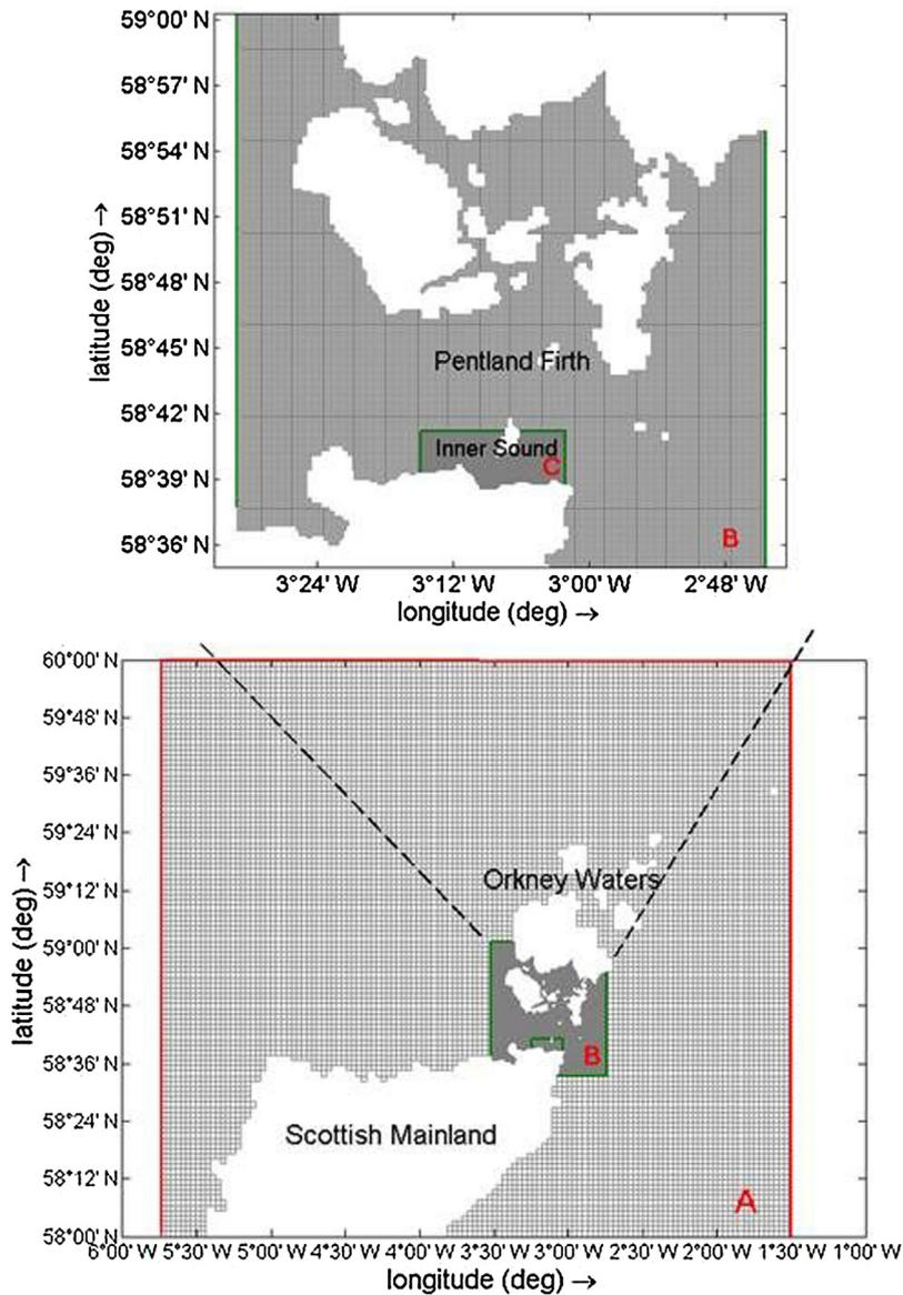
Fig. 2. Multi-scale computational domain set up. A: Large scale model covering the entire continental shelf (2 km × 2 km), B: Pentland Firth model (200 m × 200 m), C: Inner Sound channel model (66 m × 66 m). Red lines denote the open boundaries and green lines denote the coupled internal boundaries used in domain decomposition process. For further interpretation of the references to color in this figure legend, the reader is referred to the web version of this article.)
