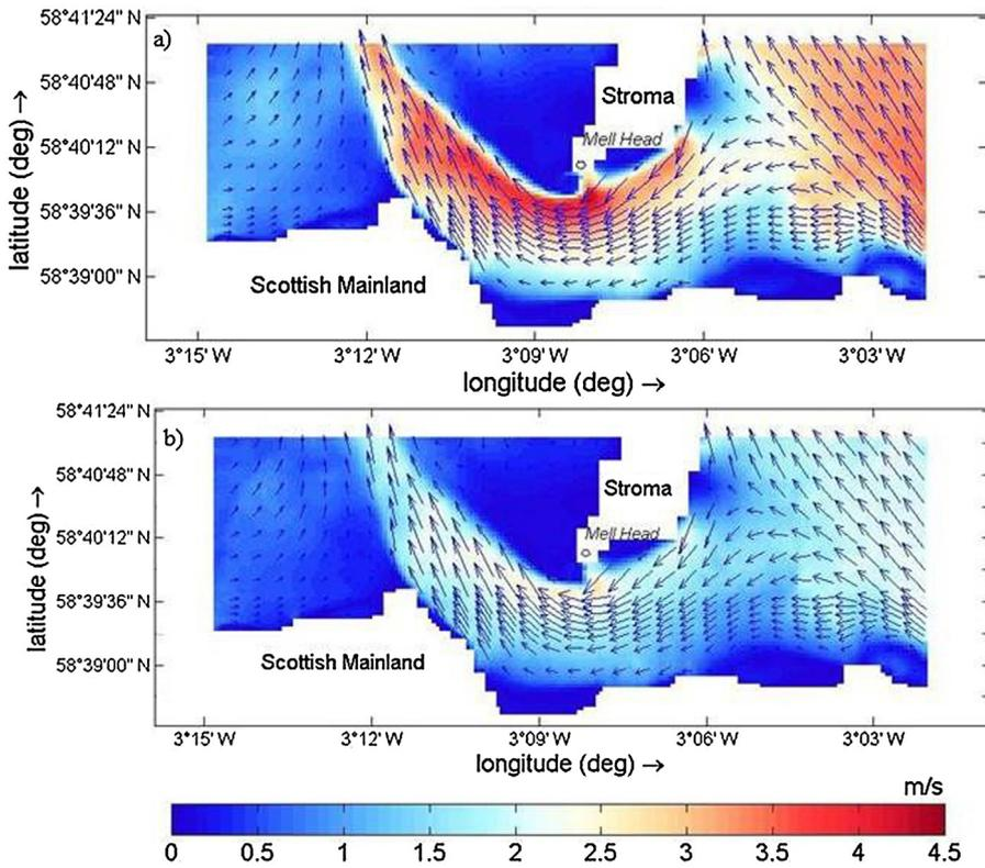
Fig. 9. Horizontal velocity (m/s) at the a) surface and b) bottom layer, at maximum spring ebb tide (04/10/2001 03:20) inside the Inner Sound channel. The colour bar indicates the magnitude of velocity and arrows indicate velocity direction.
