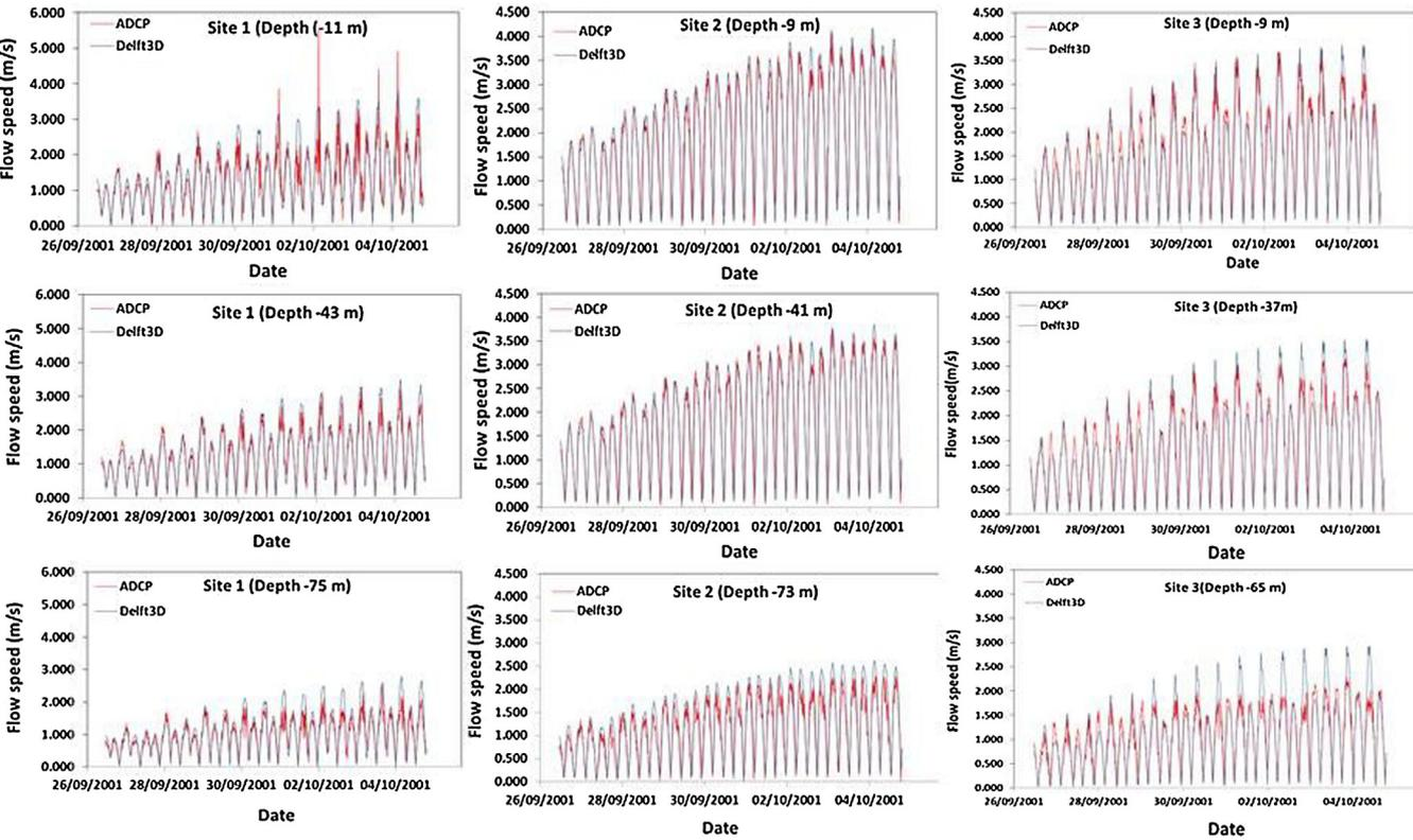
6. Comparisons of horizontal current velocity (m/s) time-series at three depths below the mean water surface, between measured and modelled flows over a full neap (09/2001)–spring (04/10/2001) tidal cycle, for the selected Delft3D flow key parameters.
