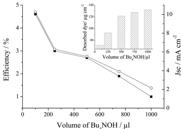
Fig. 1  $\eta$ ,  $J_{sc}$  and dye loading for a TiO<sub>2</sub> device fast dyed with N719 (1 ml, 2.8 mM) and desorbed with varying volumes of 4 mM Bu<sub>4</sub>NOH. Efficiency shown as black squares and  $J_{sc}$  as open circles. Inset shows dye loading versus volume of Bu<sub>4</sub>NOH.
