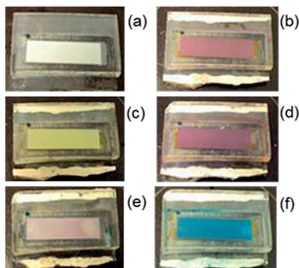
Fig. 2 DSC devices showing colour changes (a) before dyeing, (b) after N719 dyeing, (c) after N719 desorption – the yellow colour is due to I<sub>3</sub><sup>-</sup>/I<sup>-</sup> electrolyte, (d) after N719 re-dyeing, (e) after partial desorption of N719 and (f) after re-dyeing with SQ1.
