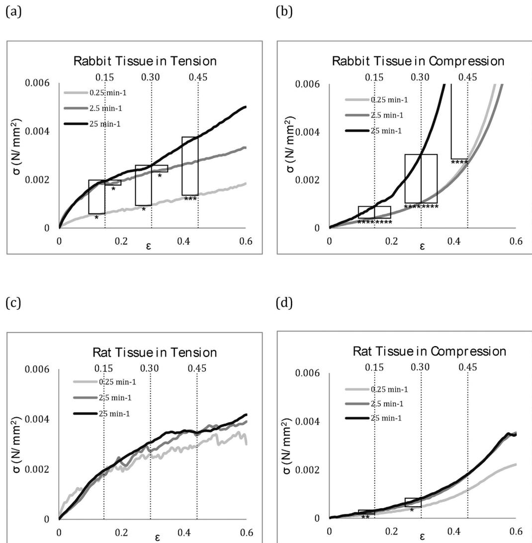
**Figure 1.** Mechanical test data for rabbit tissue under (a) tension and (b) compression; and rat tissue under (c) tension and (d) compression. Average data is presented with significance evaluated between strain rates: \* $P < 0.05$ , \*\* $P < 0.01$ , \*\*\* $P < 0.005$  and \*\*\*\* $P < 0.0001$ .
