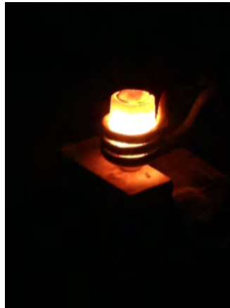
Figure 2.1: Induction melting of the Al_2CoCrFeNi HEA in a boron nitride crucible. The synthesis is performed in an Ar-filled glove box.
