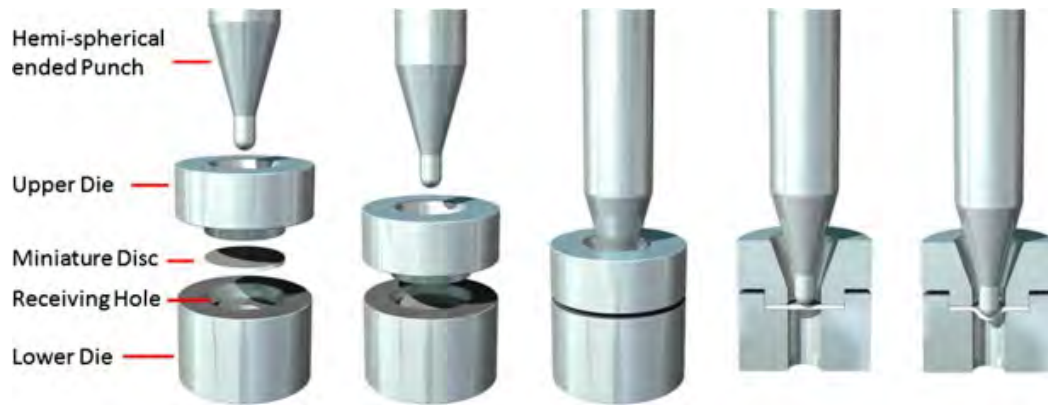
Figure 2.11: Schematics of disc retention and SP technique application [240].
