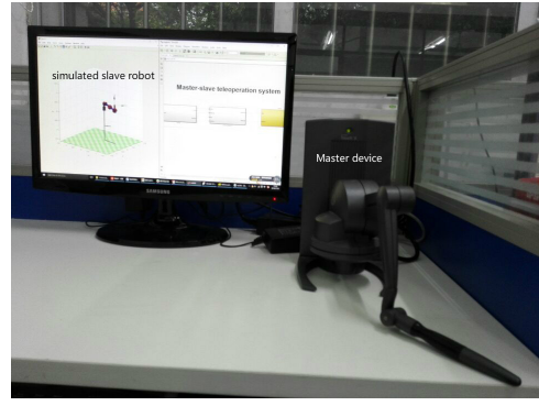
Fig. 8. The experiment platform of the master-slave teleoperation system [photo take at South China University of Technology].
