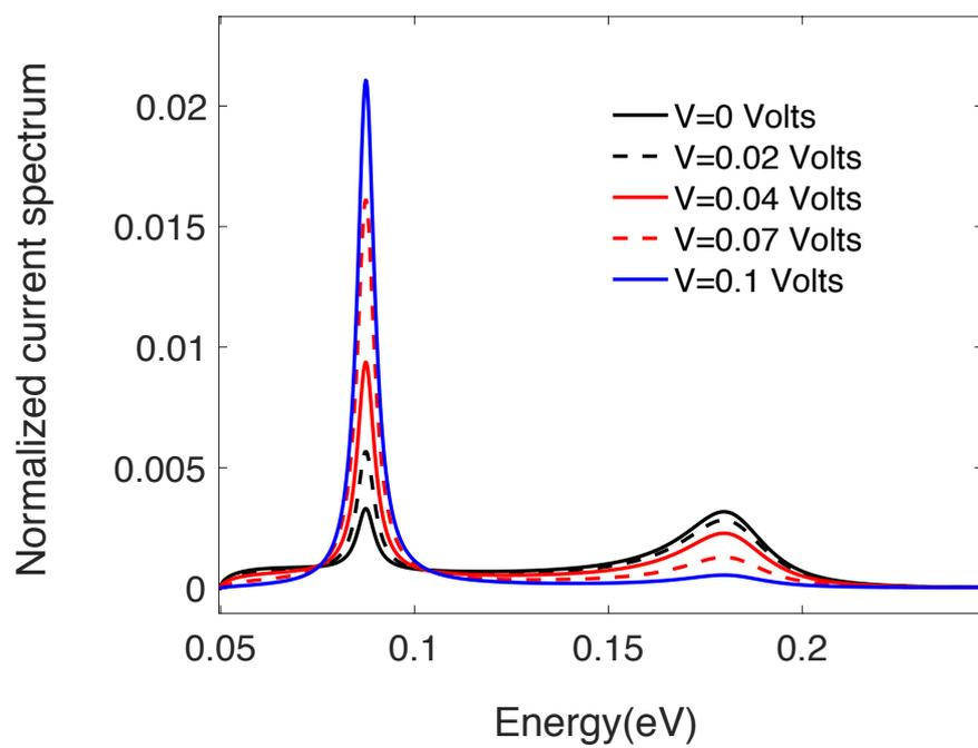
Fig. 4. The normalized current spectrum (when 2pGF is considered) for different voltages and considering ballistic transport.
