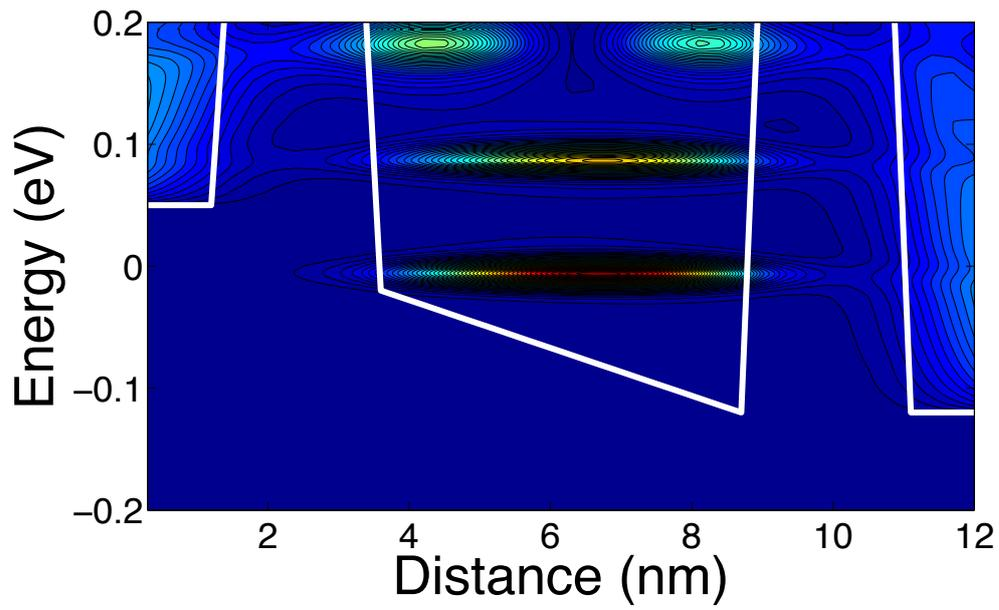
Fig. 6 LDOS for intermediate well occupation ( $0 < \text{occupation} < 2$ ). For an electron interaction coupling strength of  $0.001 \text{eV}^2$ . The two poles of the LDOS are shown simultaneously in the GR function.
