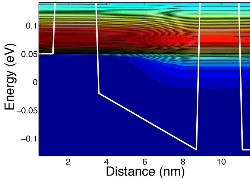
Fig 3. Current spectra through the nanostructure. The current is continuous through the structure and spread towards the right due to the inelastic scattering. The broadening of the distribution on the drain is due to inelastic phonon scattering.
