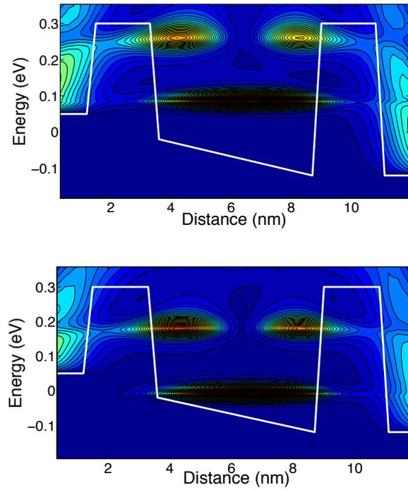
Fig.1 Upper panel: The LDOS including 2pGF. Lower panel: The LDOS without considering the 2pGF, when the electron occupation in the well is 2.
