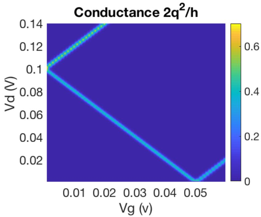
Fig. 10. Conductance as a function of gate and drain bias. Only part of the Coulomb Blockade stability diagram is shown.
