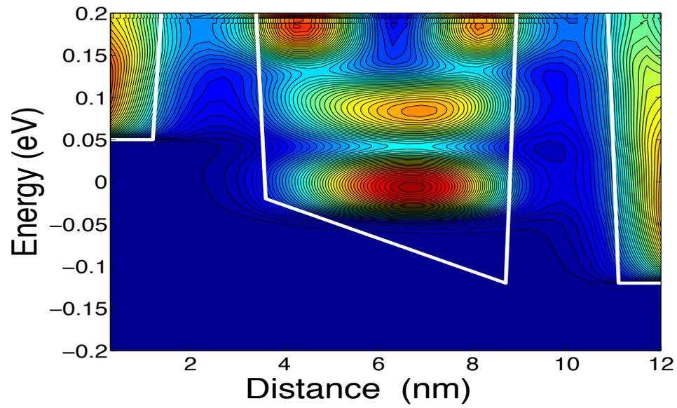
Fig. 7. LDOS for intermediate well occupation ( $0 < \text{occupation} < 2$ ). For an electron interaction coupling strength of  $0.01 \text{eV}^2$ . The large broadening of the energy levels are a result of strong electron-phonon coupling
