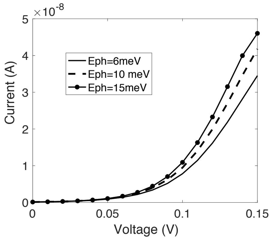
Fig. 8 The current voltage characteristics for different phonons energies including 2pGF.
