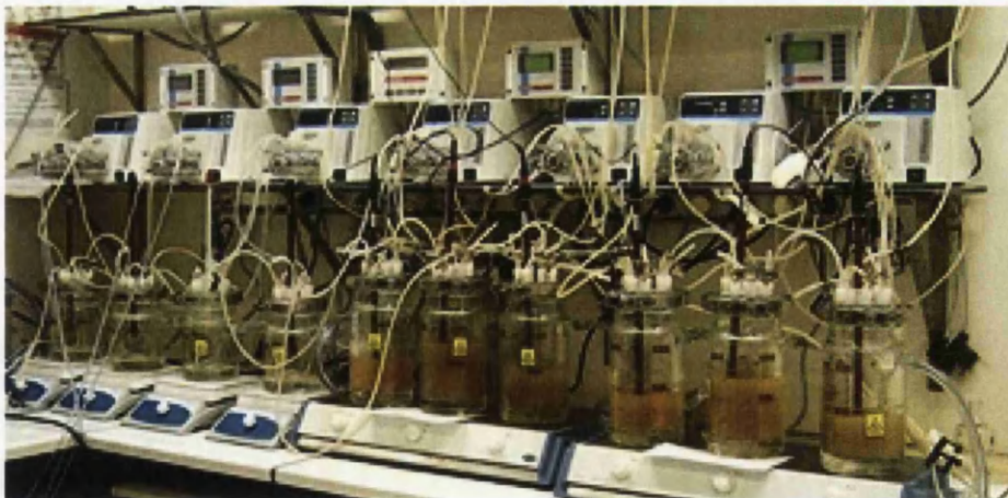
Figure 2.2: TWINSHIME System: two SHIME systems are run in parallel (Source from http://www.prodigest.eu ).
