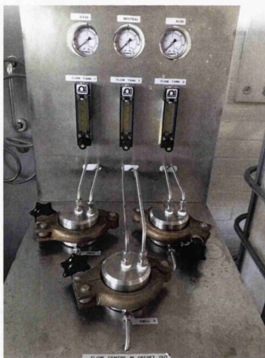
Figure 7.4 Microfiltration Cells of the integrated system
