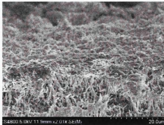
Figure 5.33 SEM micrographs of 0.22 \mu\text{m} PVDF membranes after filtering solution with 1g resin/L: (a)surface (b)cross section
