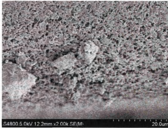
Figure 7.23 SEM micrographs of the 0.22 \mu m used PVDF membranes for regeneration step using 0.2M NaOH: (a)surface (b)cross section
