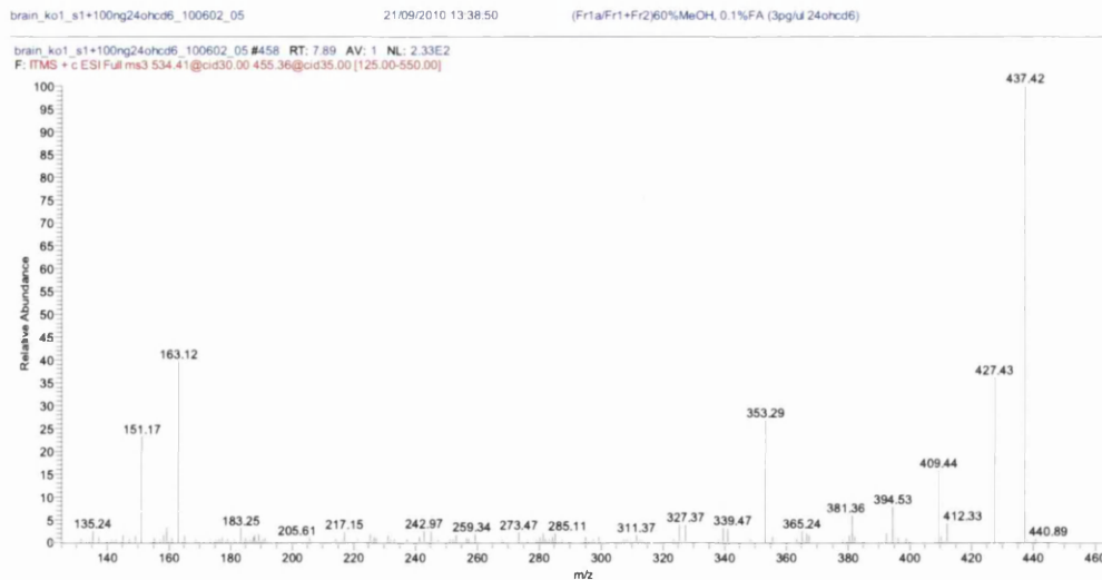
Figure 5.8. MS 3 spectrum of peak eluting at 7.49 min identified as GP-tagged 24R-hydroxycholesterol
