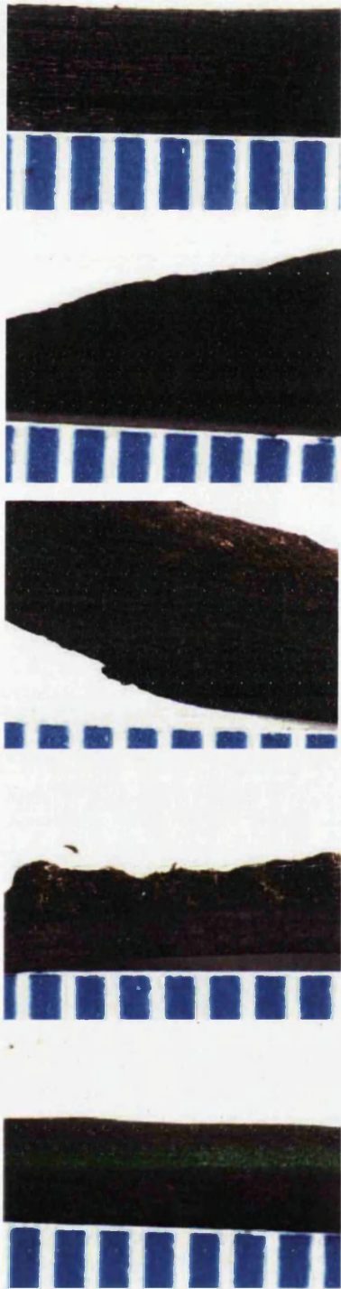
Figure 4.10: Stereomicroscope images of Picea biochars (for scale, blue marks are at 1 mm intervals)
