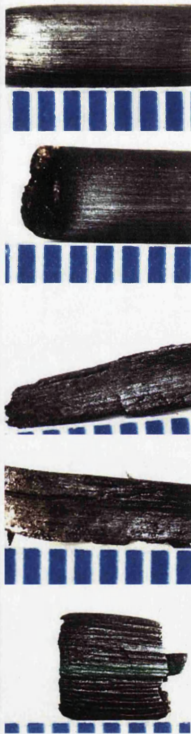
Figure 4.8: Stereomicroscope images of Miscanthus biochars (For scale, blue marks are at 1 mm intervals)
