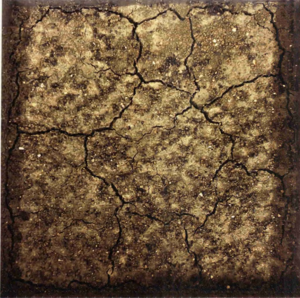
Figure 7.11: A surface crust formed by drying of a surface seal in a 300 x 300 mm soil plot with a biochar content of 25 g kg -1
