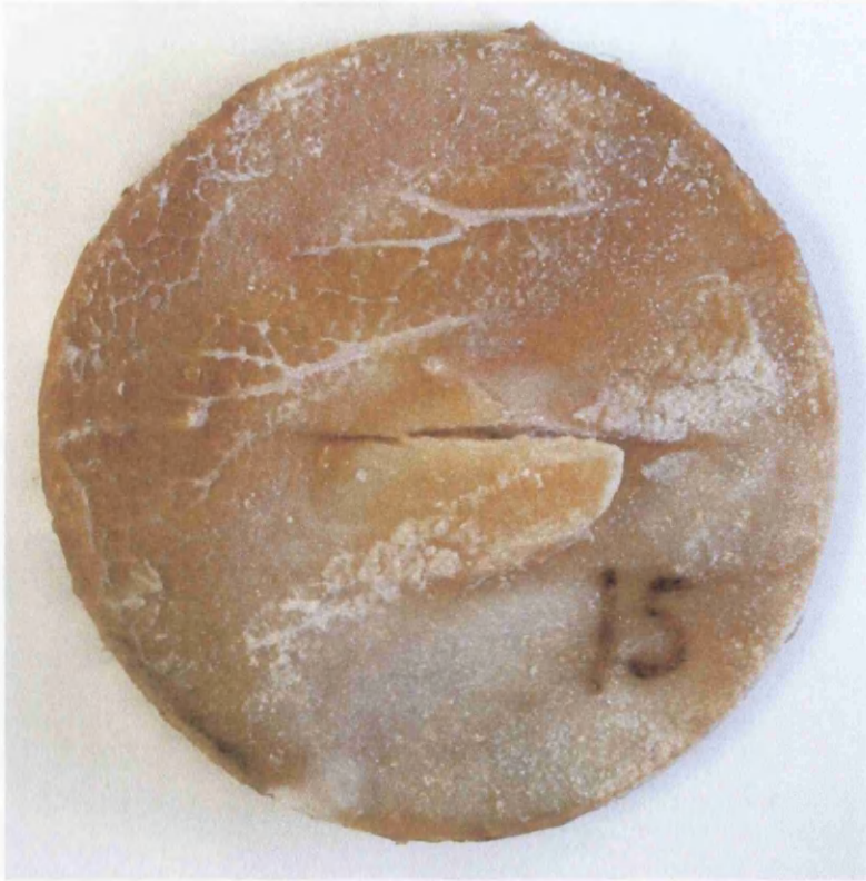
Figure 4.38 Failed disk sample showing failure type e): complex cracking from diametric crack
