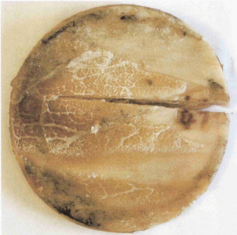
Figure 4.35 Failed disk sample showing failure type b): single diametric crack through the disk
