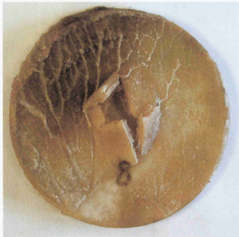
Figure 4.39 Failed disk sample showing failure type f): complex cracking from the edge of the indenter
