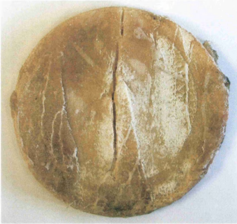
Figure 4.34 Failed disk sample showing failure type a): single diametric crack
