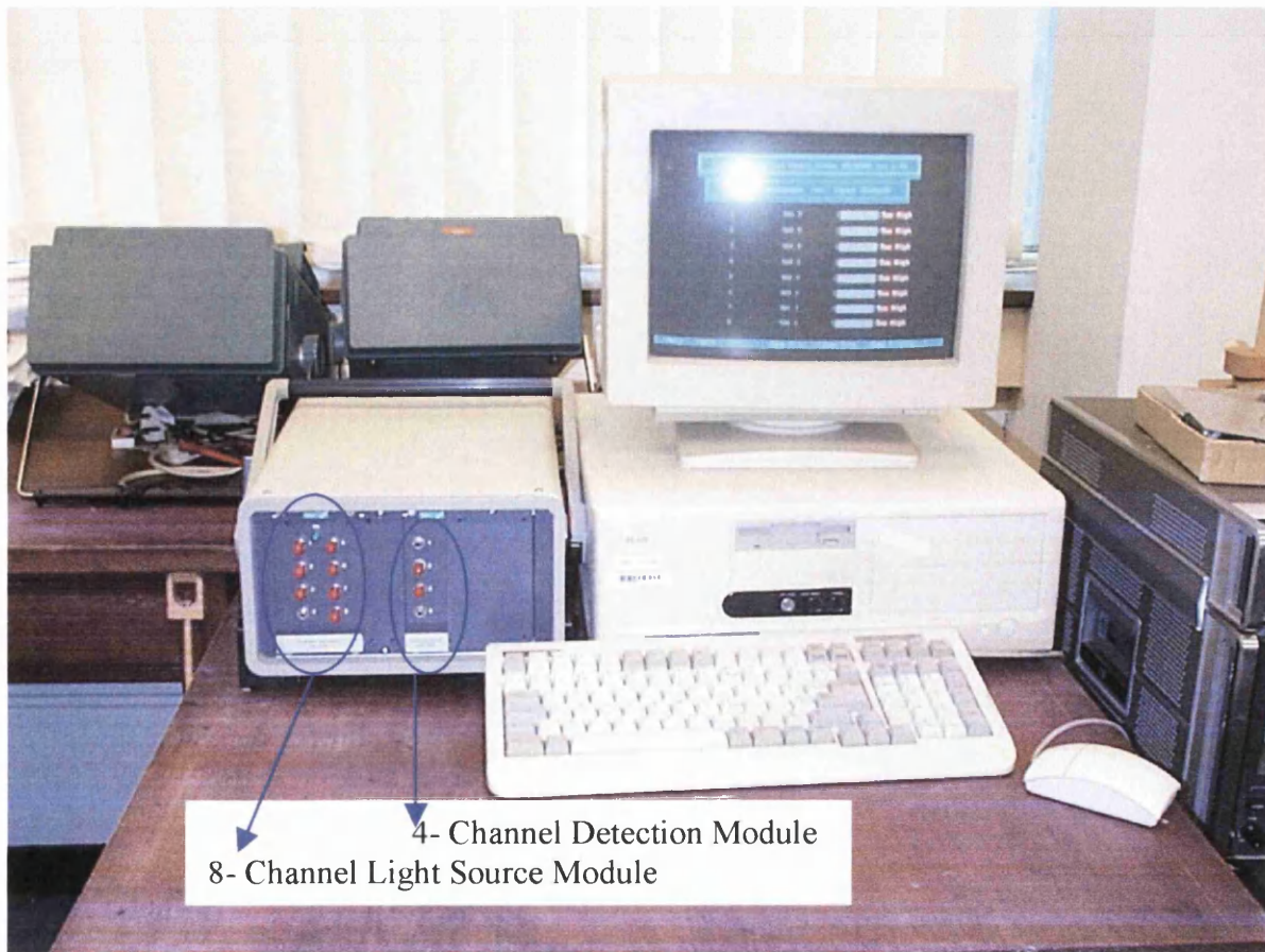
Figure 4.6 - Optical Strain Gauge System
