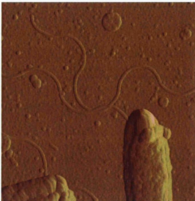
Figure 3-18: AFM amplitude image showing cells and flagella, scan size is 4.4 \times 4.4 \mu\text{m} .
