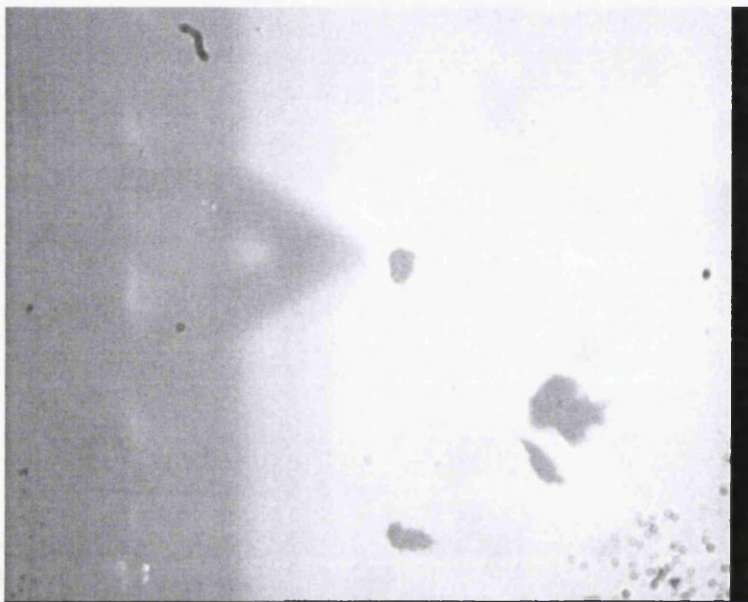
Figure 2-3: Graphite powder particle shown on glass slide before capture by prepared cantilever. The cantilever is out of focus but visible due to proximity to the surface, with the target graphite particle just in front of the apex of the cantilever. This particle was measured as 5\mu\text{m} by 7.5\mu\text{m} on the image by comparison with the graticule image.
