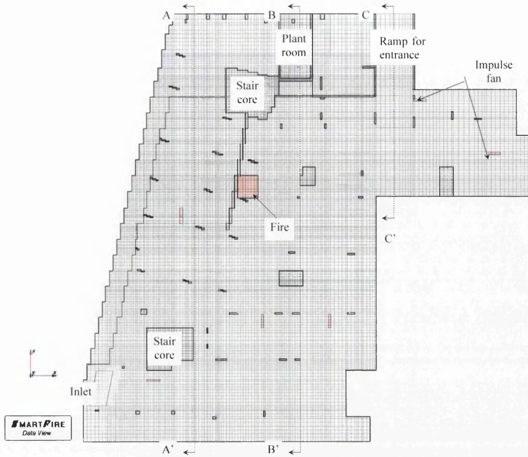
Figure 6.48 – Plan view of the underground car park.
