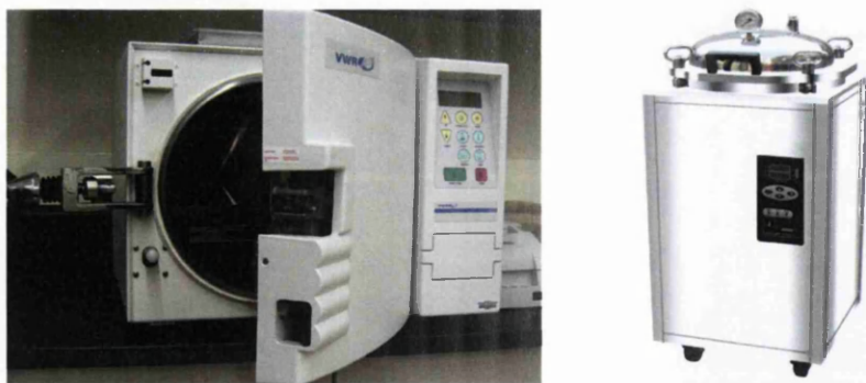
Figure 20. Shows a typical desktop lab autoclave (left), high-pressure upright autoclave (right).
