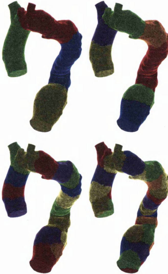
Figure 3.8: Parallel Test 2. METIS decomposition of the aorta for each parallel run. a) 4 Patch b) 8 Patch c) 16 Patch d) 32 Patch
