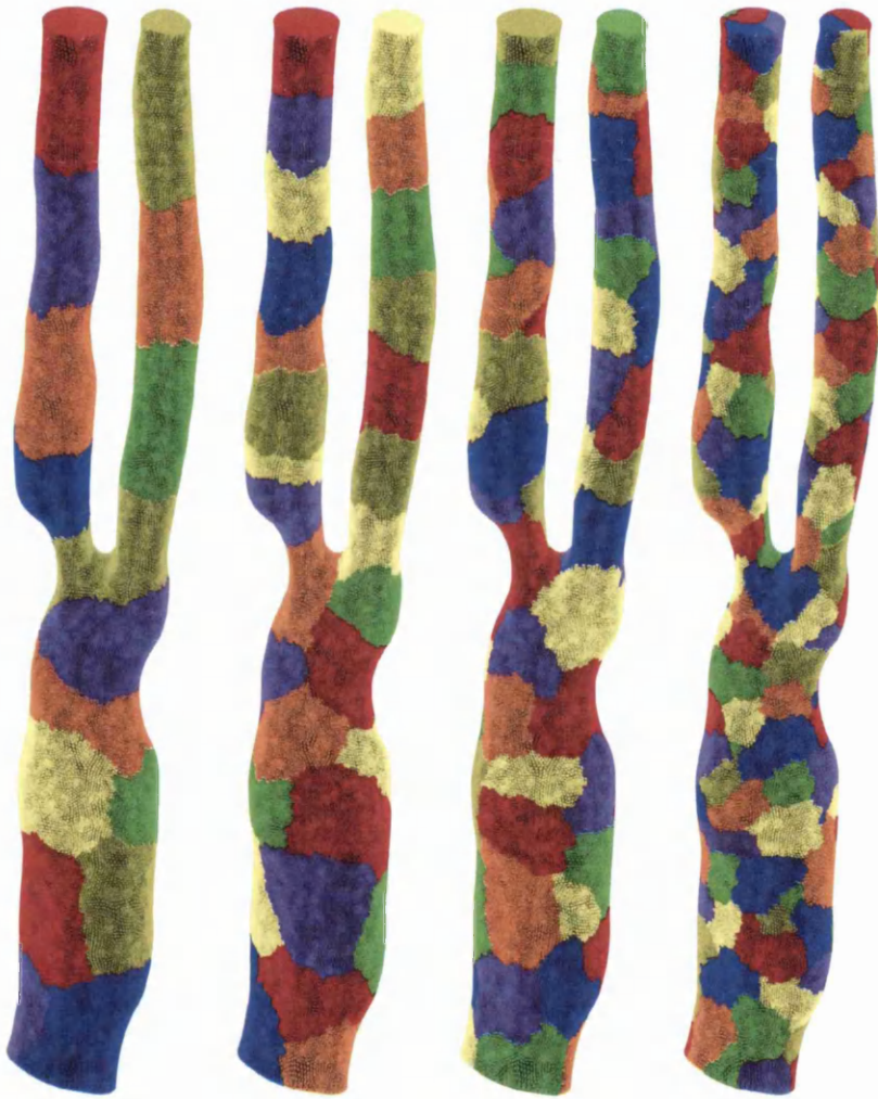
Figure 3.10: Parallel Test 3. METIS decomposition of the carotid for the parallel runs. a) 16 Patch b) 32 Patch c) 64 Patch d) 256 Patch
