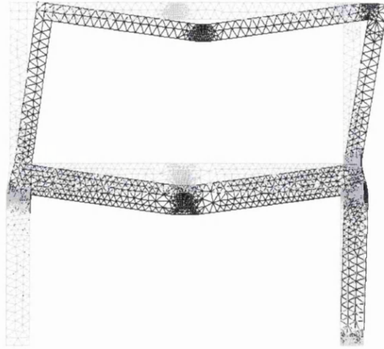
Figure 6.59 Collapse mechanism for the reticular frame W
