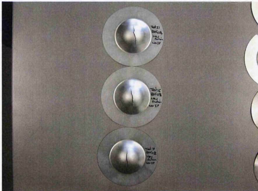
Figure 3.36. Set of three 50 halterwidth bank successfully stretch until failure.
