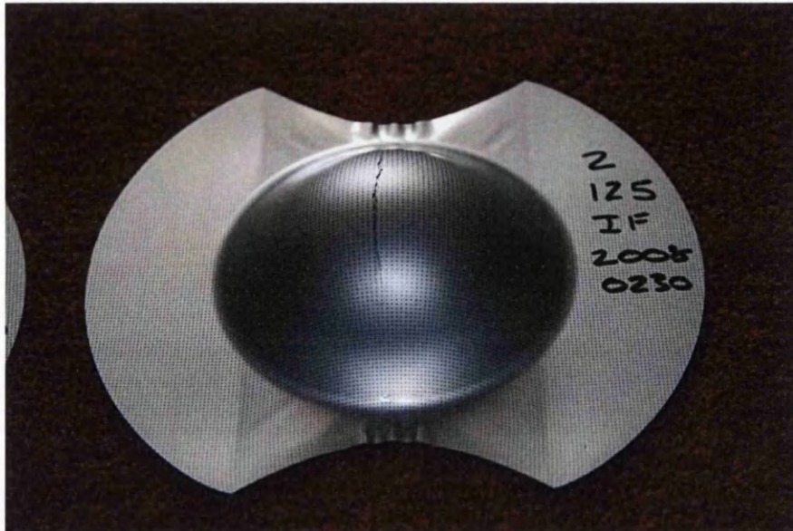
Figure 4.17. Experimental results showing wrinkling in halterwidth blank 125
