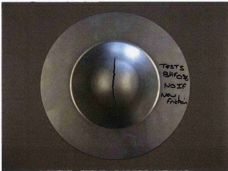
Figure 3.31. 166 halterwidth formed blank using the new lubrication method.
