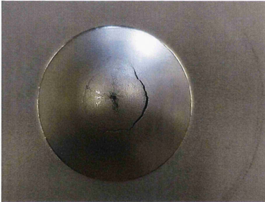
Figure 3.18, material T57CA with no lubrication produces a circular crack.
