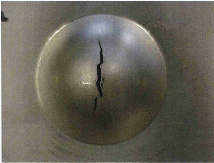
Figure 3.19, material T57CA with Vaseline spray lubrication produces a centre crack.
