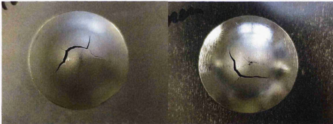
Figures 3.5 and 3.6 showing materials T59 CA and DR 550 CA that cracked perpendicular to the rolling direction respectively.
