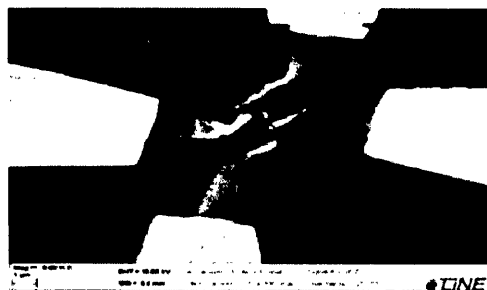
Figure 5.17: SEM image of the fabricated device using ZnO nanowire 6 (NW6).
