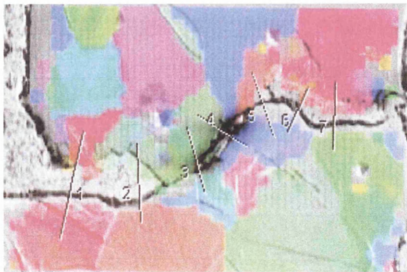
Figure 4.0c The top images correspond to the bottom half of the matched fracture specimen shown in the image above, which has been sectioned to a depth of 80 microns. It can be seen that there is a correlation in the colours shown by the orientation maps
