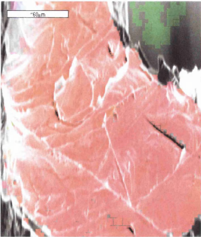
Figure 4.3a,b Crystal Orientation Maps taken from fracture surface facets
