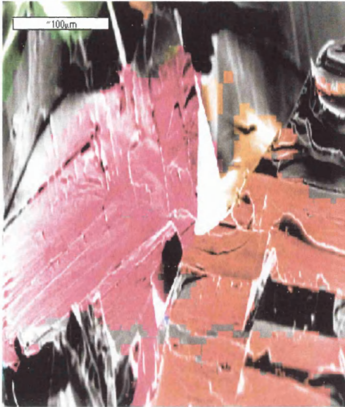
Figure 4.3a,b Crystal Orientation Maps taken from fracture surface facets
