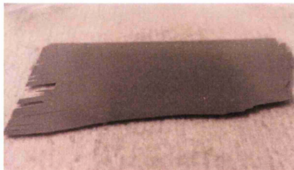
Figure 5.21: Textured silicon foil after metallic contact removal
