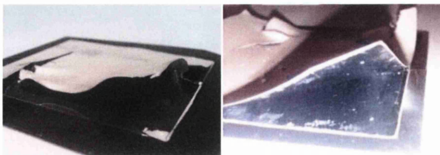
Figure 5.15: (a) Polished wafer after firing process, (b) Textured wafer after firing process
