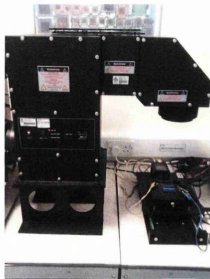
Figure 4.13: Oriel solar tester equipment used to measure cell performance
