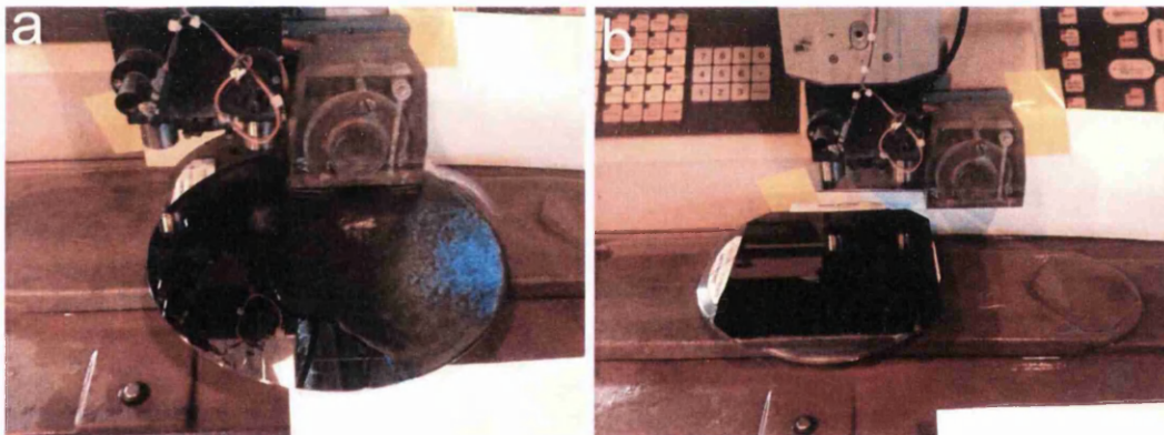
Figure 4.9: Dicing of a circular 200mm silicon wafer (a), into a 156mm x 156mm pseudo square (b)
