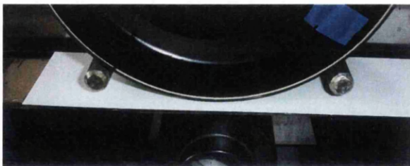
Figure 8.2.2: Close up view of the point of contact between the printing plate, substrate, substrate holder and impression cylinder. Note how the substrate is driven by pressure between the two cylinders.
