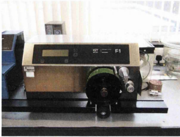
Figure 8.2.1: Photograph of the IGT F1 flexographic printability tester used for device production.
