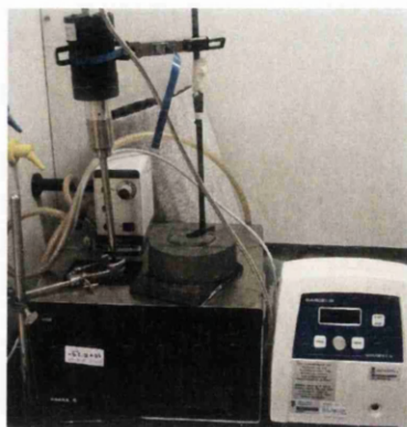
Figure 3.2.1: Bandelin Sonopuls 3100 ultrasonic homogeniser probe setup in the configuration described in section 3.2.1.3.
