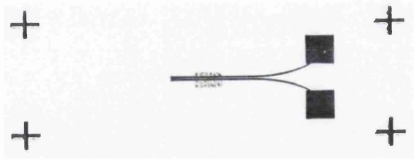
Figure 10.5.2: Optical scan of representative print of electrode structure printed above the CNT layer. Printing direction was left to right.
