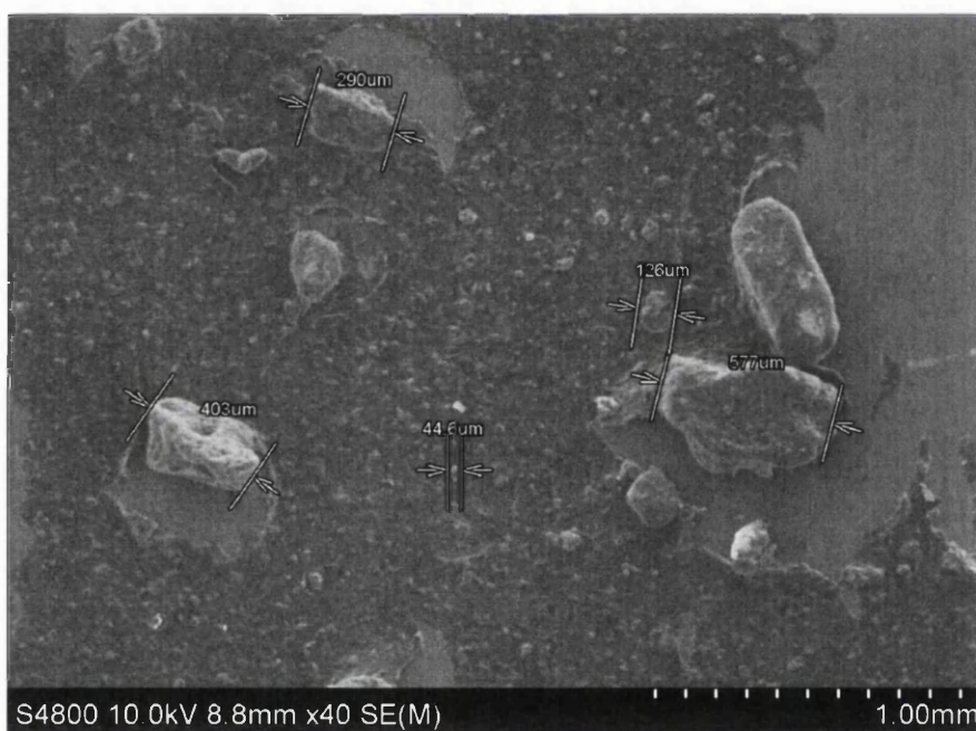
Figure 2.2.1: SEM image highlighting typical agglomeration sizes in an untreated commercial SWCNT powder.
