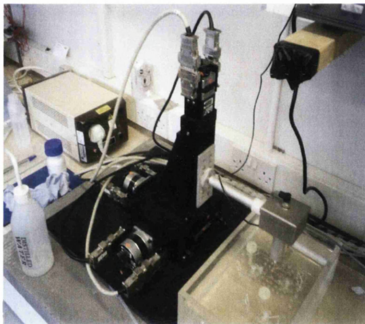
Figure 3.4 The experimental setup of Scanning Vibrating Electrode Technique. Source Swansea University website*.
