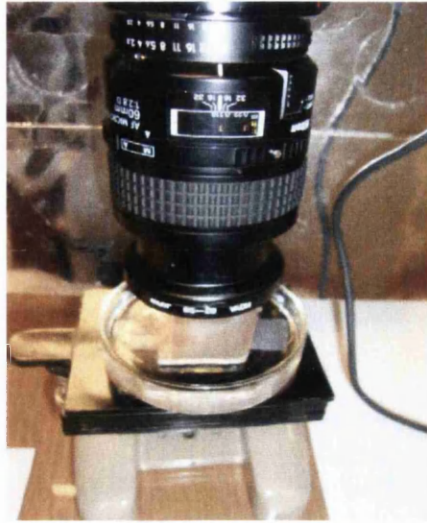
Figure 3.1 Experimental setup of time lapse photography with the Petri-dish in the bottom and the camera lens directly over it.
