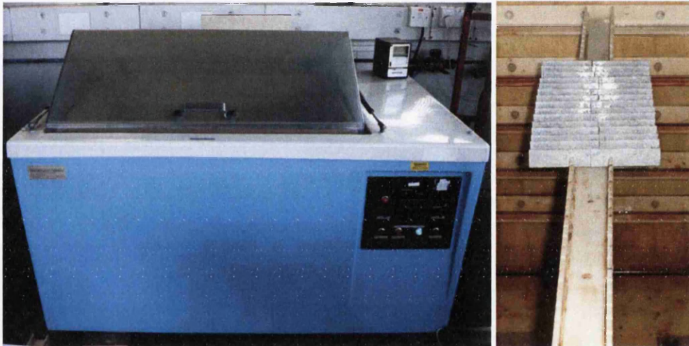
Figure 17 Humidity cabinet used for long-term weathering studies. The sets of lap joints were positioned horizontally in slotted racks.
