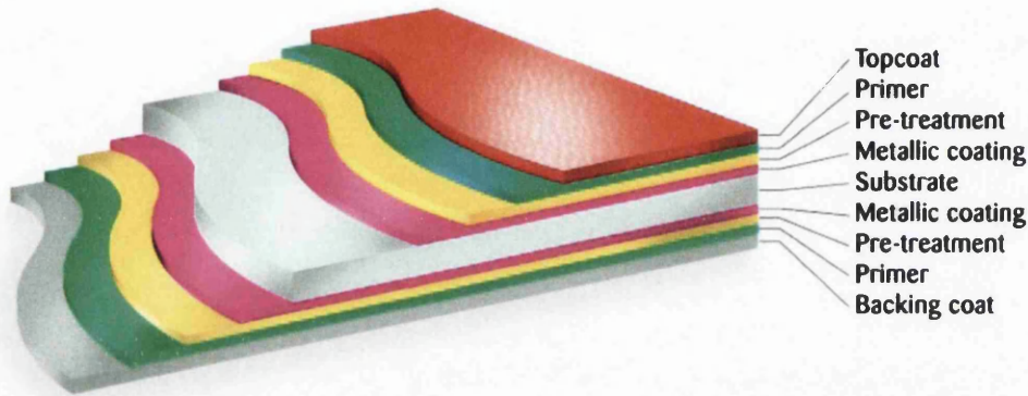
Figure 12 The protective layers of organic coated steel products [59].
