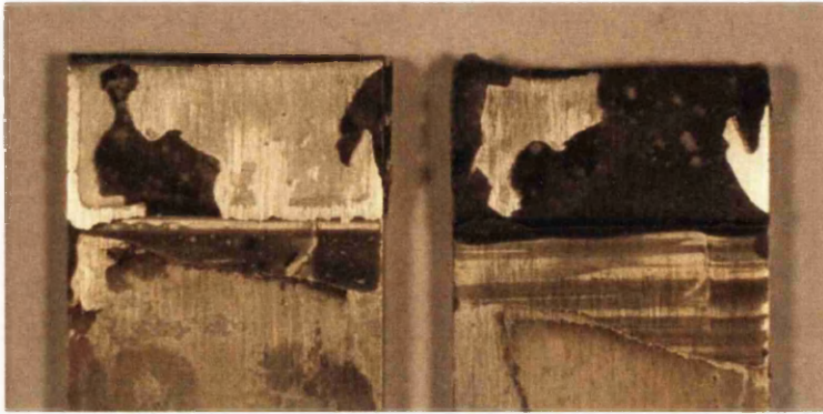
Figure 50 Aluminium interfacial and corrosion failure.
