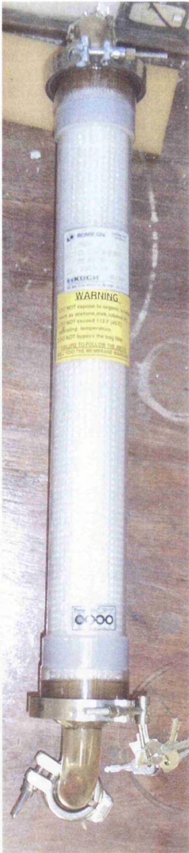
Figure 4-5 Koch Hollow fibre PAN Membrane Module
