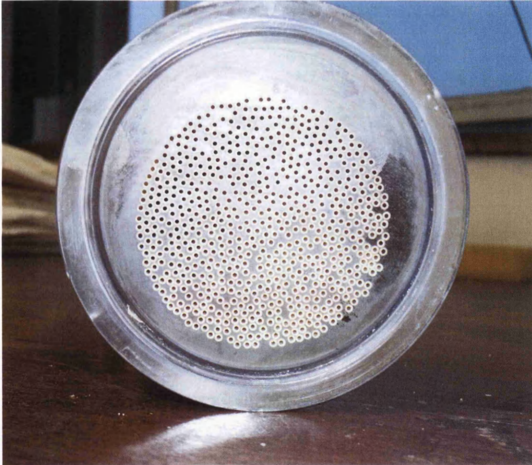
Figure 4-4 End view of Hollow fibre module (PAN)
