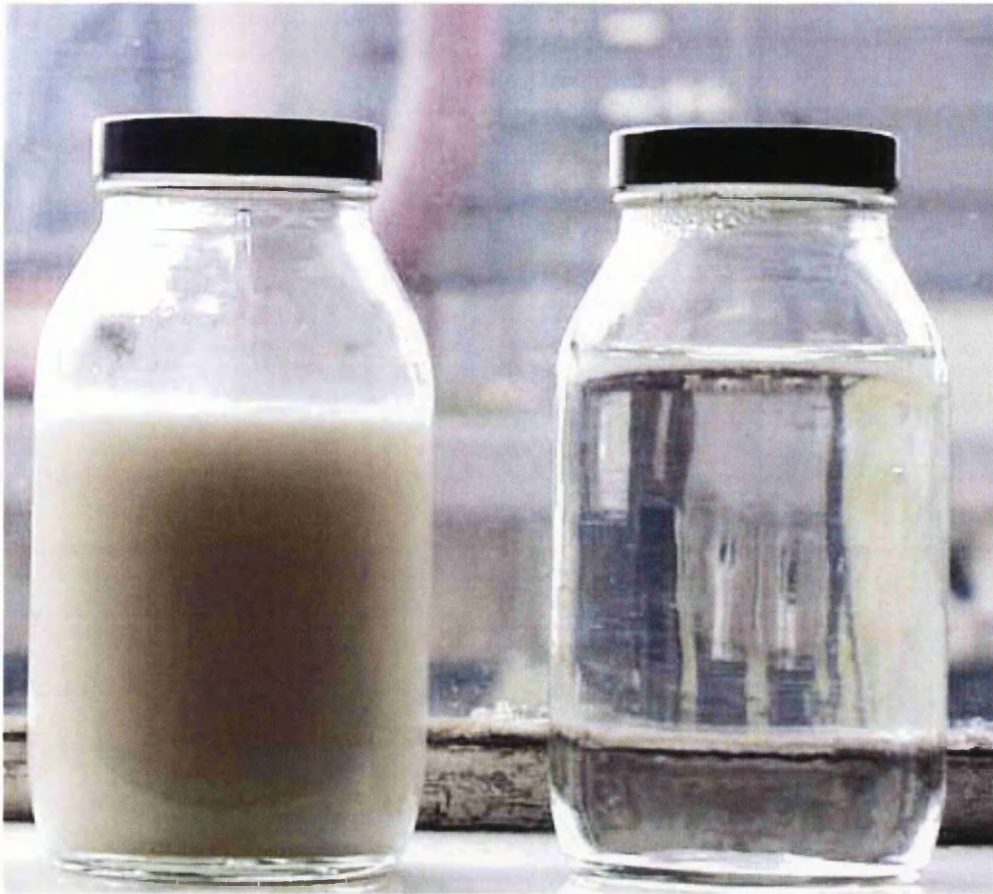
Figure 5-1 Example of the Typical Emulsion (on left) next to a Permeate Sample
