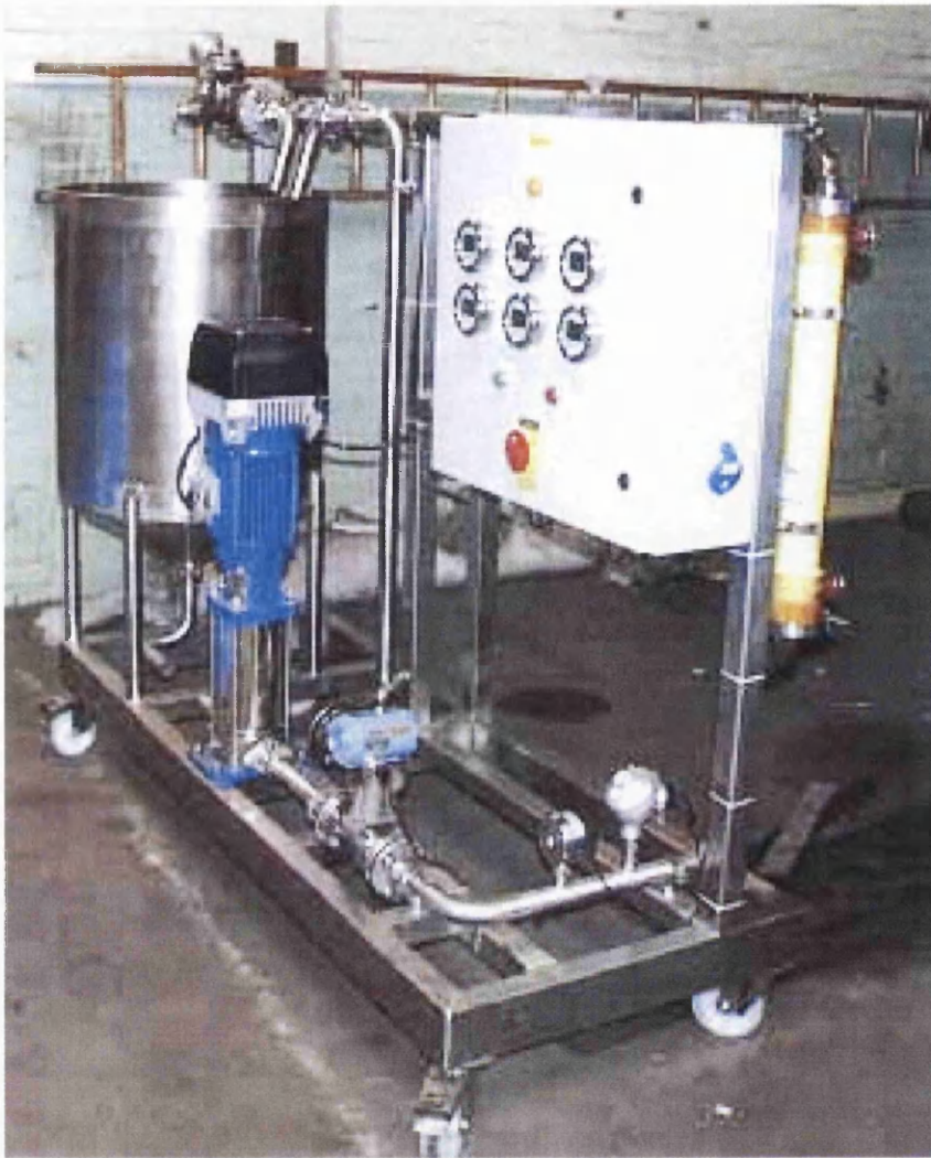
Figure 4-1 Pilot Rig showing PS Hollow fibre Membrane
