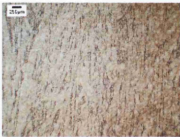
Figure D.1: Microstructure of brass specimen, magnification \times 16
