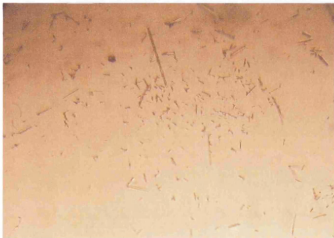
Figure 5.8 An optical microscope image of nanobelts deposited on silicon wafer before photolithography process was started.
