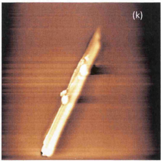
Figure 6.8 EFM images of silicon n-type nanowire 2 taken at a scan size of 6.5\mu\text{m} \times 6.5\mu\text{m} and a tip height of 50nm with a tip bias of (a) -10V, (b) -8V, (c) -6V, (d) -4V, (e) -2V, (f) 0V, (g) +2V, (h) +4V, (i) +6V, (j) +8V and (k) +10V.
