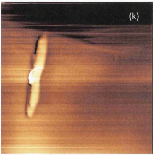
Figure 6.10 EFM images of silicon p-type nanowire 1 taken at a scan size of 4.5\mu\text{m} \times 4.5\mu\text{m} and a tip height of 50nm with a tip bias of (a) -10V, (b) -8V, (c) -6V, (d) -4V, (e) -2V, (f) 0V, (g) +2V, (h) +4V, (i) +6V, (j) +8V and (k) +10V.
