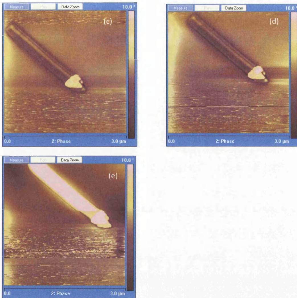
Figure 6.1 3\mu\text{m}\times 3\mu\text{m} size EFM scans of zinc oxide nanowire and gold catalyst particle taken at a tip height of 50nm with (a) tip bias of -2V, (b) tip bias of -4V, (c) tip bias of -6V, (d) tip bias of -8V and (e) tip bias of -10V.
