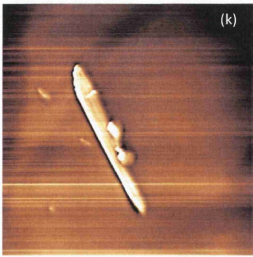
Figure 6.6 EFM images of n-type silicon nanowires 1,3 and 4 taken at a scan size of 4.5\mu\text{m}\times 4.5\mu\text{m} and a tip height of 50nm with a tip bias of (a) -10V, (b) -8V, (c) -6V, (d) -4V, (e) -2V, (f) 0V, (g) +2V, (h) +4V, (i) +6V, (j) +8V and (k) +10V.
