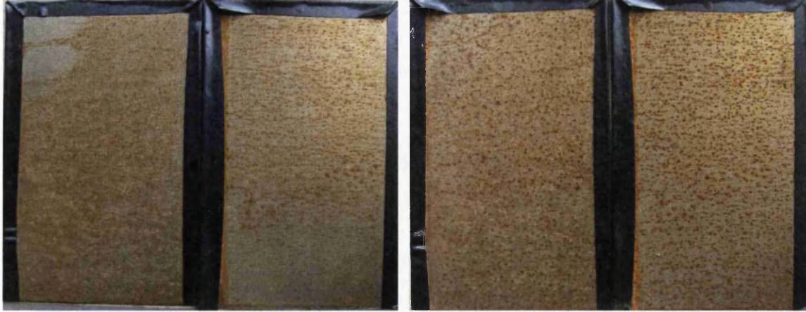
Fig 7.17 Photographic images of duplicate tests of Sample 19 held in a humidity chamber for a) 24 h and b) 2 weeks.
