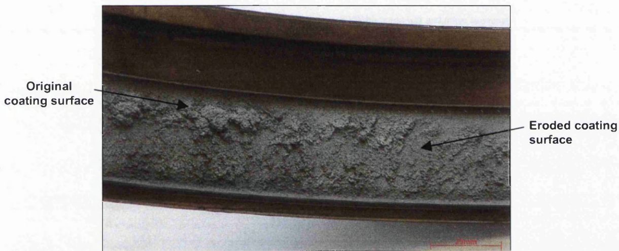
Figure 25. Erosion damaged Sherritt Gordon abradable coating
