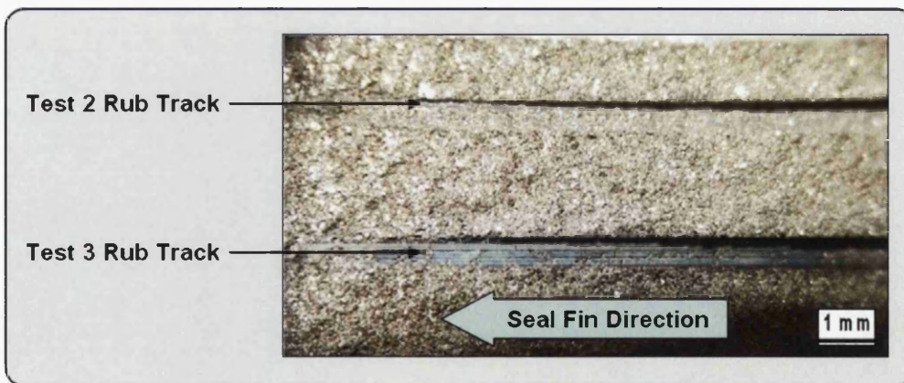
Figure 62. Rub tracks from abrasability Test 2 and Test 3.
