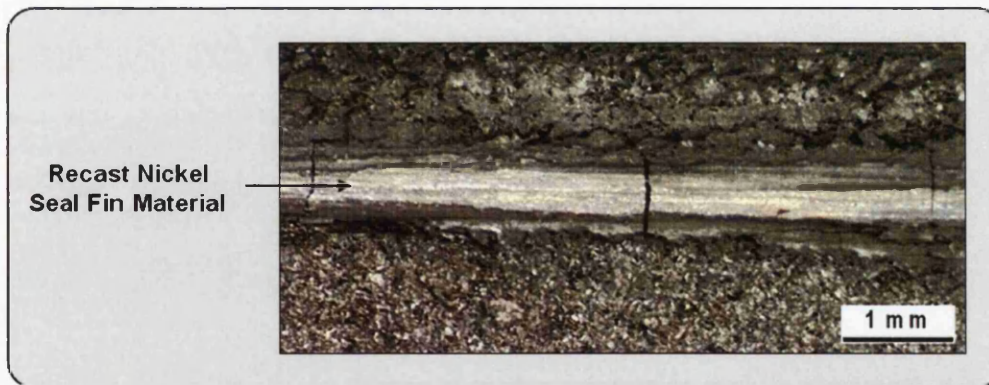
Figure 53. Seal fin transfer as a result of excessive frictional heating during engine rub
