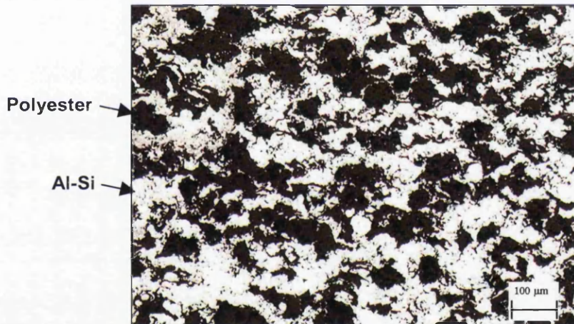
Figure 15. Microstructure of Metco 601
