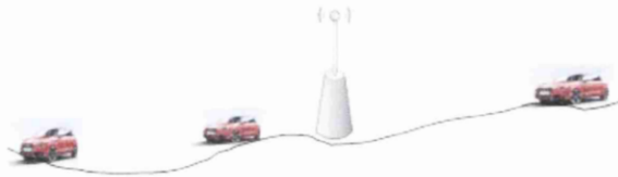
Figure 5.6: Vehicles with Short Range Communication devices drive past an 802.11 Access Point.
