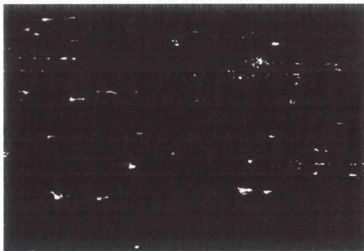
Figure 4.5: Examples of back-scatter micrographs from SEM for the side surface of AA2024-T351. The aluminium matrix appears black, and the transition metal containing intermetallics white.
