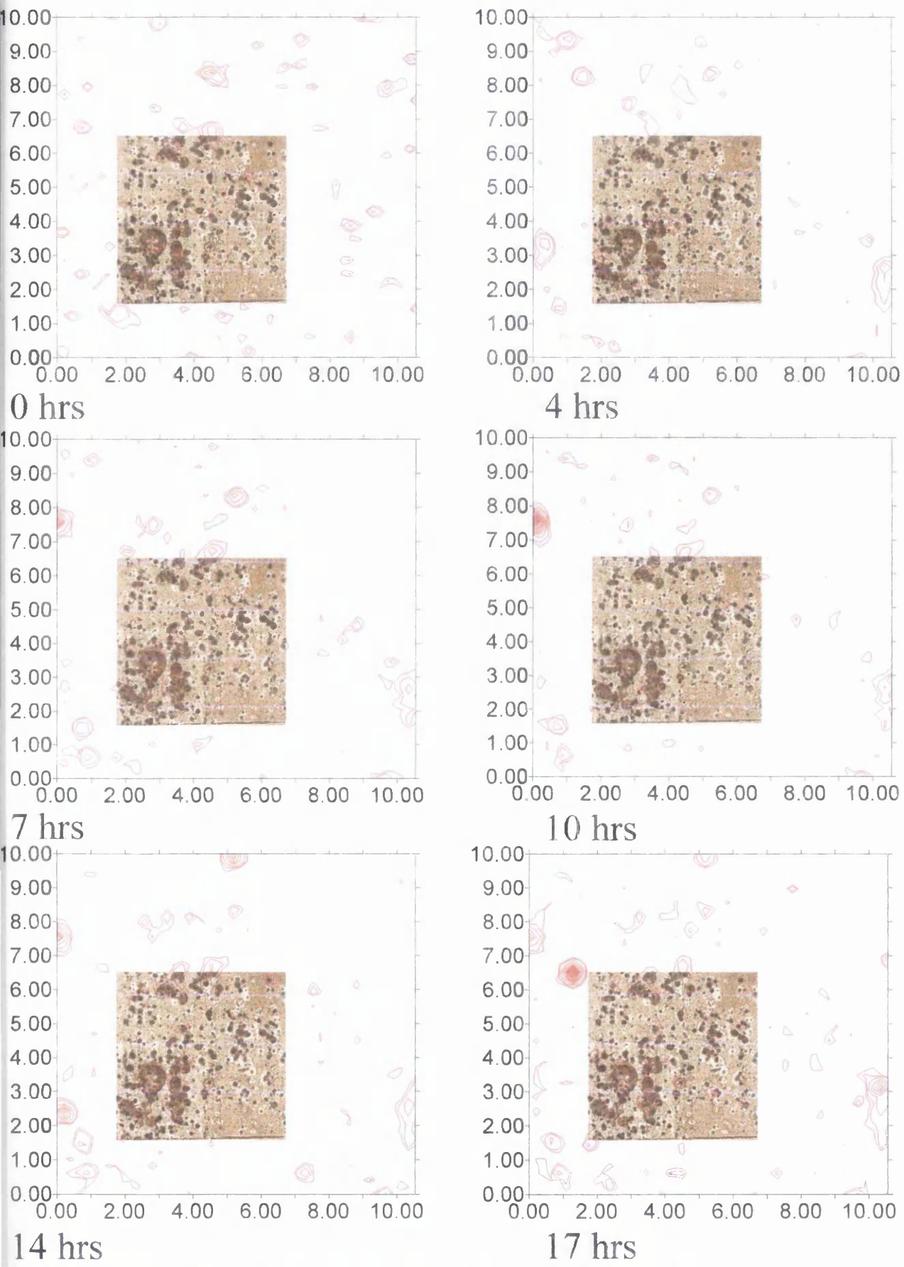
Figure 3.8: SVET data contour lines after X hours, set over in-situ image of surface after 17 hours immersion in 3.5% w/w NaCl.
