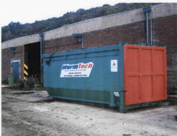
Figure 2.7 In-vessel container system designed to compost food waste
