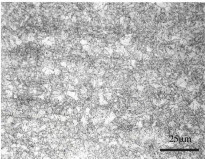
Figure 6.4. Micrographs of a 5Vt spot weld made in alloy DP800 (CE - 0.22): (d) the variation in microstructure from the edge of the nugget through to the parent material; (e) heat-affected zone microstructure.
