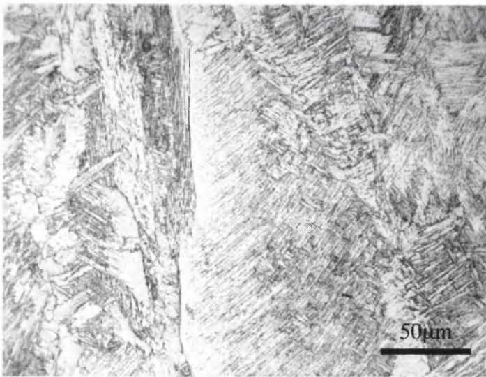
Figure 6.2. Micrographs of a 5\sqrt{t} spot weld made in alloy LCNb (CE - 0.07): (a) parent microstructure (b) macro showing shape of weld and heat-affected zone; (c) columnar grains in the weld nugget.
