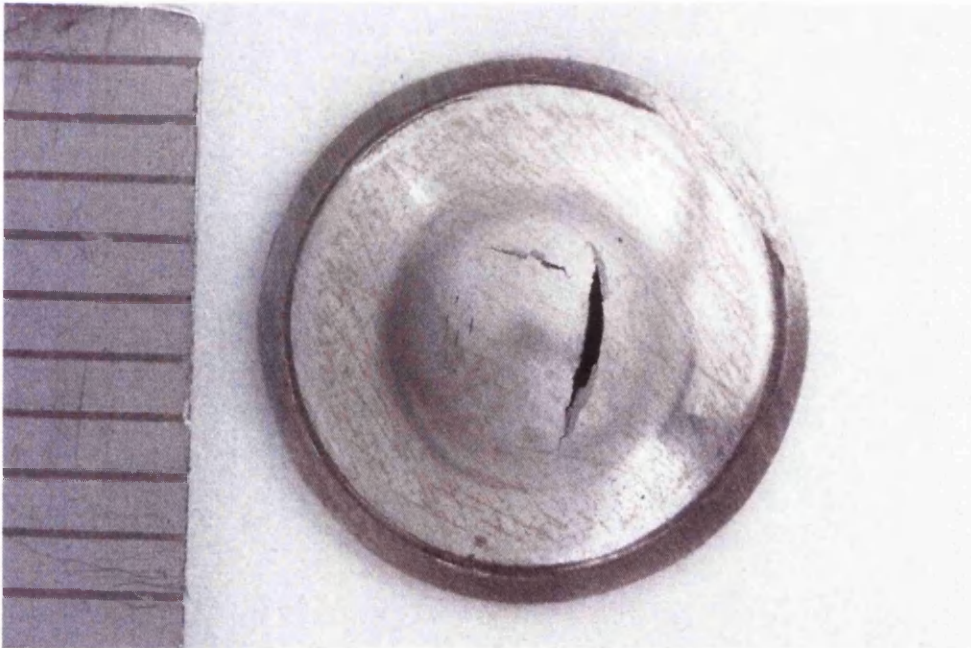
Figure 5.15. Photograph of the failure of a 0.5mm thick disc of DP800 after testing at 1\text{mm}\cdot\text{min}^{-1} . (Scale at side is mm)
