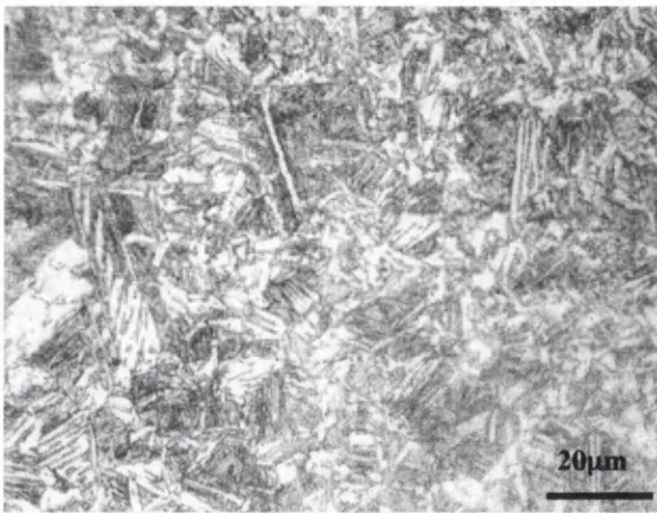
Figure 6.20. Typical micrographs from alloy DP1000 (CE – 0.24) after normalizing and cooling using a Gleeble 3500. Cooling rate: (j) 1950°C/s.
