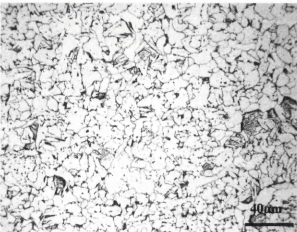
Figure 6.18. Typical micrographs from alloy DP600 (CE – 0.14) after normalizing and cooling using a Gleeble 3500. Cooling rate: (d) 5°C/s; (e) 10°C/s; (f) 20.1°C/s.
