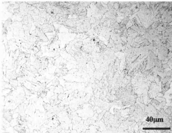
Figure 6.16. Typical micrographs from alloy LC (CE = 0.04) after normalizing and cooling using a Gleeble 1500. Cooling rate: (g) 26.7°C/s; (h) 26.6°C/s; (i) 392°C/s.
