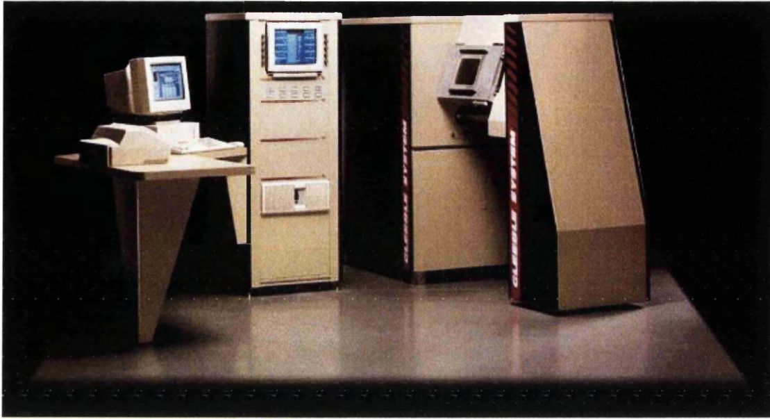
Figure 4.3. General photograph of a Gleeble 3500 thermomechanical simulator.
