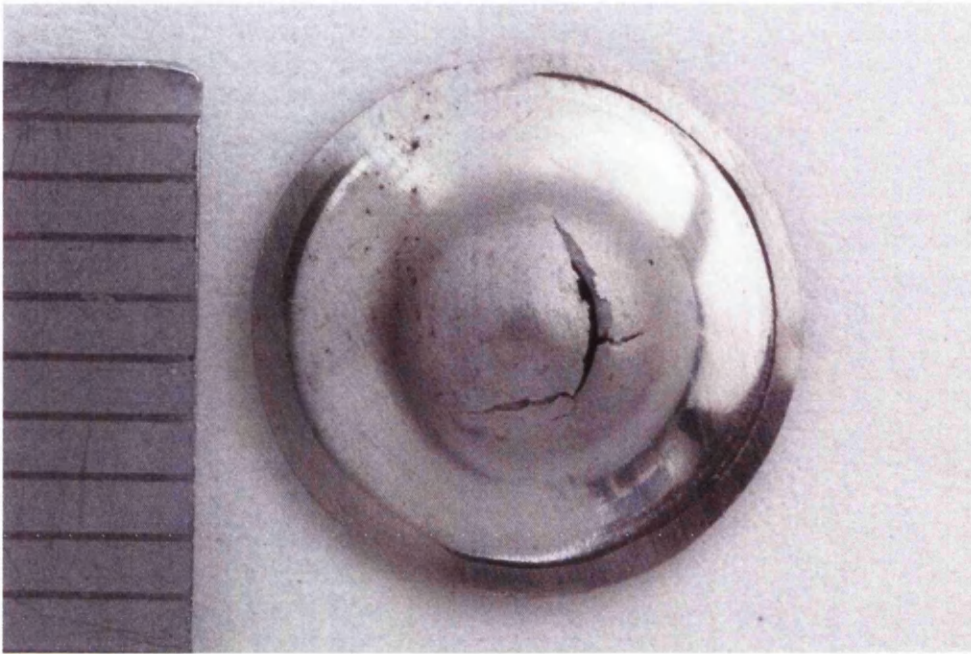
Figure 5.18. Photograph of the failure of a 0.5mm thick disc of DP800 after testing at 3\text{mm}\cdot\text{min}^{-1} . (Scale at side is mm)
