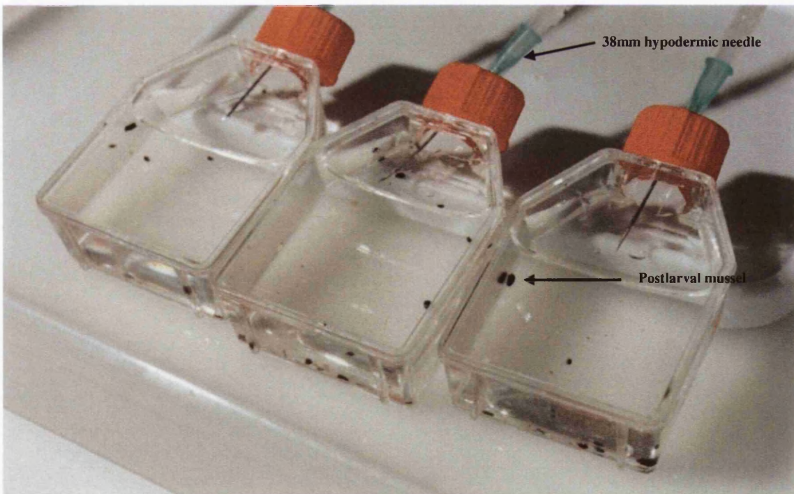
Figure 4.2. Tissue culture vessel postlarval exposure method: detail showing hypodermic needles entering through the vessel lid to aerate the media.
