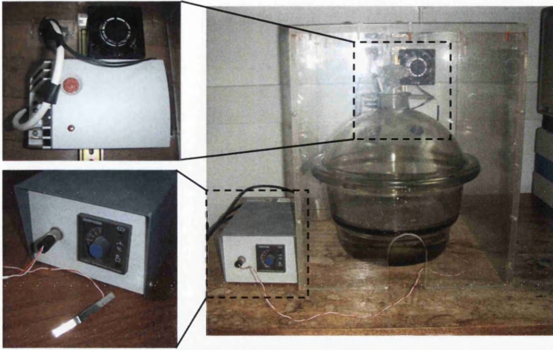
Figure 3.3 Photographs showing the accelerated applied acid test humidity chamber and thermostatically controlled air bath equipment.
