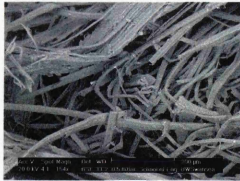
Fig. 5.11: Fracture surfaces of tensile tested samples with low resin content
