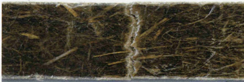
Fig. 5.45: Fracture surface of a hemp fibre composite sample in fatigue testing
