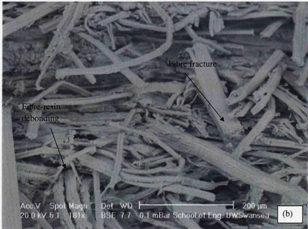
Fig 5.9: SEM micrographs of fracture surfaces of tensile tested hemp fibre reinforced polyester samples
