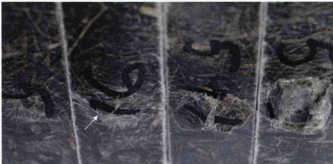
Fig. 6.29: Macrographs of distal face of 1% alkalised fibre composite samples with increasing impact energy levels from left to right
