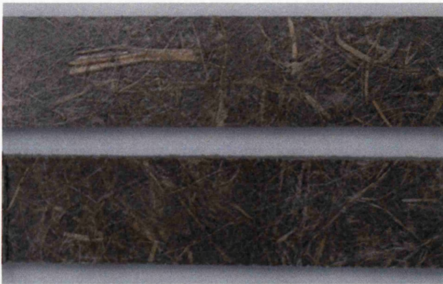
Fig. 5.55: Comparison of sample fatigue tested at stress level 50% of UTS (top) with untested sample (bottom)
