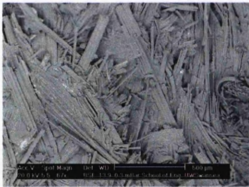
Fig. 6.36: SEM micrographs of the surface of 5% alkalised fibre composite sample that endured 10^6 cycles, \sigma= 34 MPa.
