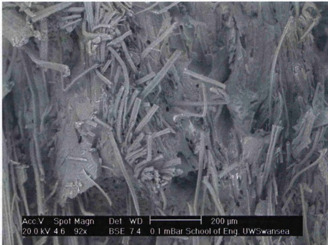
Fig. 6.42: SEM micrographs of fracture surface of tensile tested sample of plasma treated fibre composites
