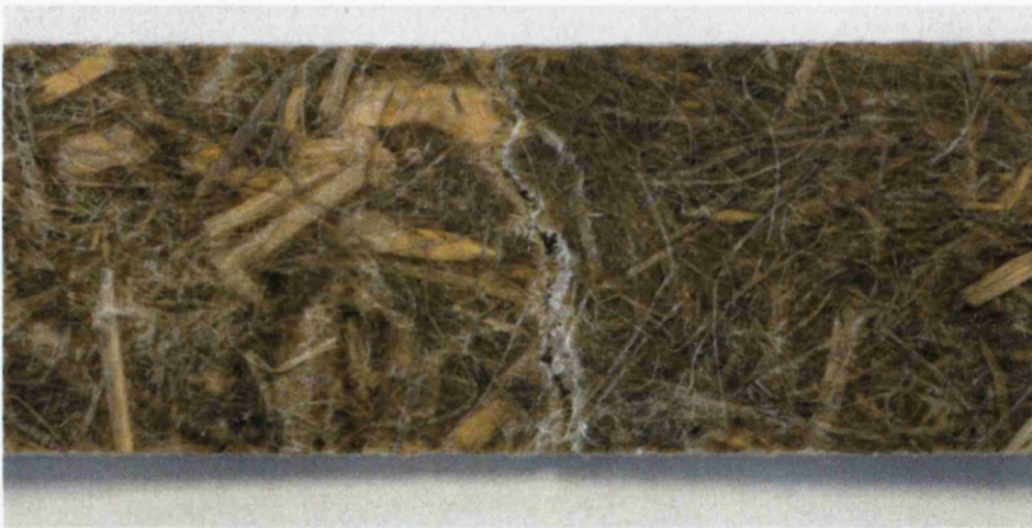
Fig. 5.5: Fracture surface of a hemp-polyester sample in tensile testing
