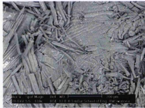
Fig. 6.36: SEM micrographs of the surface of 5% alkalised fibre composite sample that endured 10^6 cycles, \sigma= 34 MPa.
