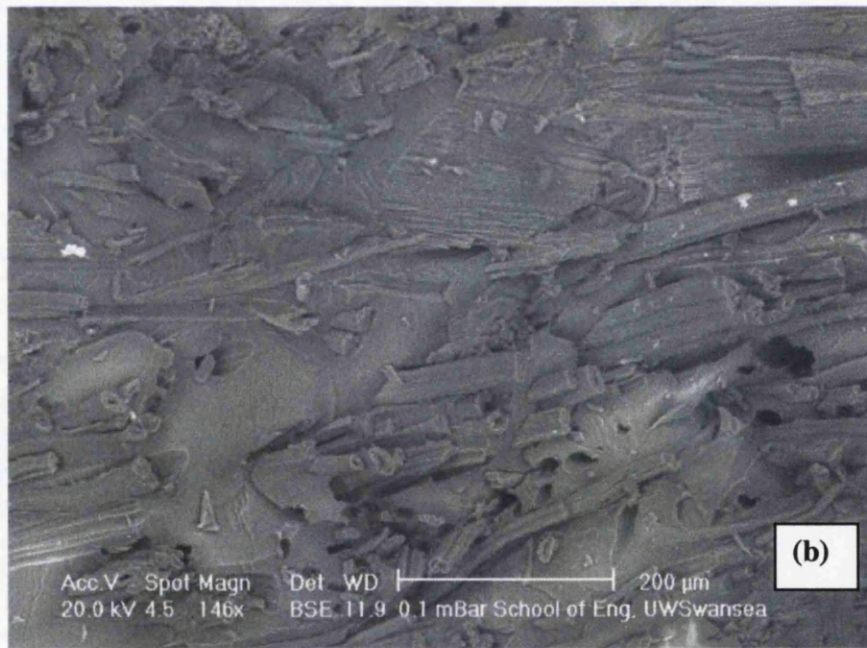
Fig. 6.22: SEM micrographs of fracture surfaces of (a) 1% alkalisated and (b) 10% alkalisated fibre composites after tensile testing
