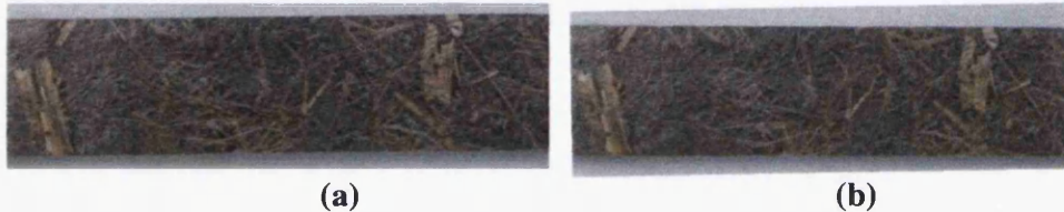
Fig. 5.8: Surface of hemp composite sample before testing (a), and after tensile testing (b), at stress=37 MPa, strain=0.8%
