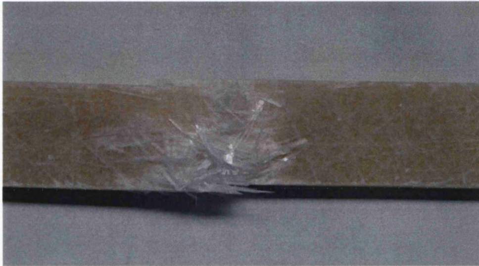
Fig. 5.14: Fracture surface of tensile tested CSM glass-polyester sample
