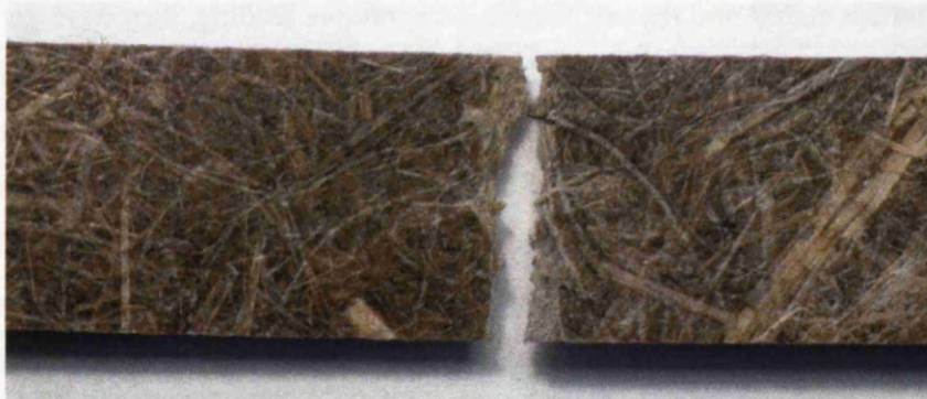
Fig. 5.72: Fractured sample in tension-compression fatigue
