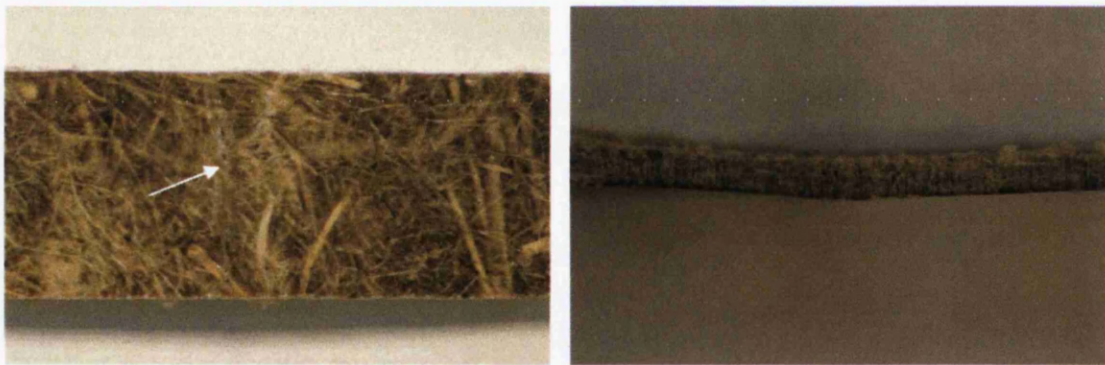
Fig. 5.73: Fracture surfaces of flexural tested sample
