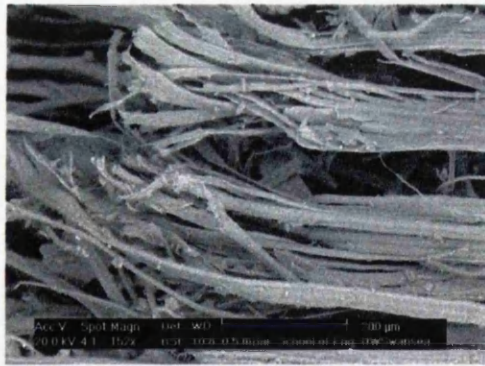
Fig. 5.11: Fracture surfaces of tensile tested samples with low resin content
