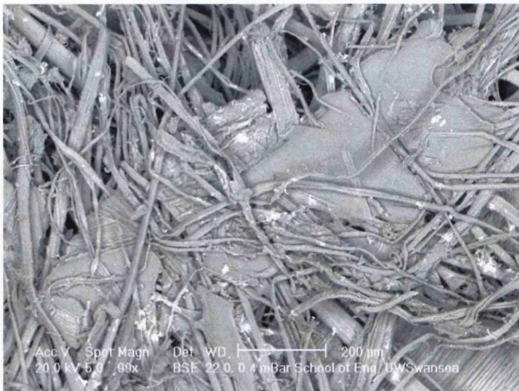
Fig. 7.22: SEM micrograph of fracture surface of fatigue tested samples pre-immersed in water
