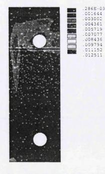
Figure 5.41 Plastic deformation of the S690 endplate
