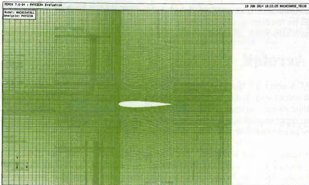
Figure 6-26- Magnified image of the structured grid for the NACA0012 aero foil at the leading edge for 70,132 elements.
