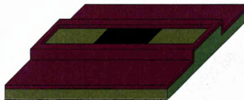
(b) Photoresist mask for metal deposition.
