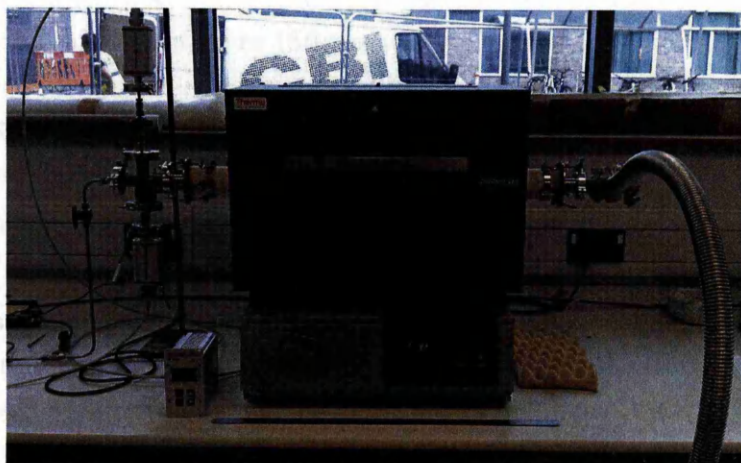
Figure 3.2: Thermo Scientific tube furnace. Gas inlet is on the left with Pirani and piezo vacuum gauges mounted on the cross piece. The vacuum hose is connected on the right.
