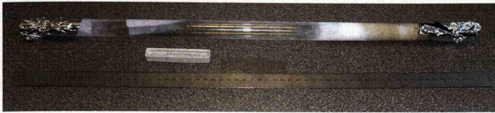
Figure 3.3: Quartz tube following growth (gas flow from left to right). An alumina source boat is also shown. Condensation of ZnO vapour is seen both upstream and downstream.
