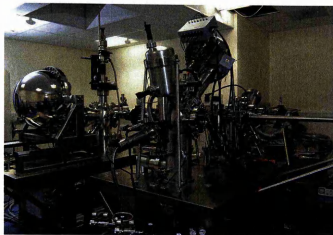
Figure 3.26: Science City Photoemission Facility, University of Warwick. The far system is for angle resolved photoemission spectroscopy (ARPES).
