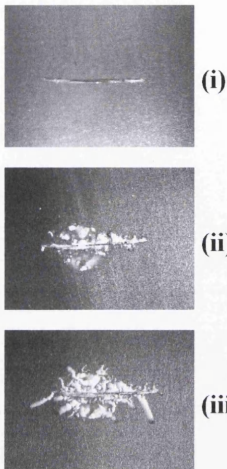
Figure 5-4 : surface appearance of 10mm penetrative defect on sample (b) (2wt% PPA) after initiation with 1.5 \mu l of 1.5mol/dm 2 aqueous acetic acid. Propagation conditions are 86%RH and 22°C. Propagation time is (i) 1 week, (ii) 3 weeks, (iii) 5 weeks.
