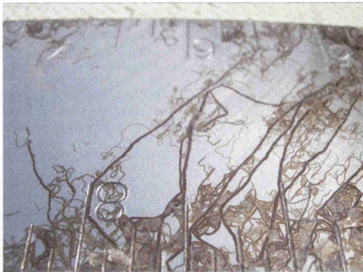
Figure 1-5 : Typical visual appearance of filiform corrosion filaments on an organically coated steel ruler
