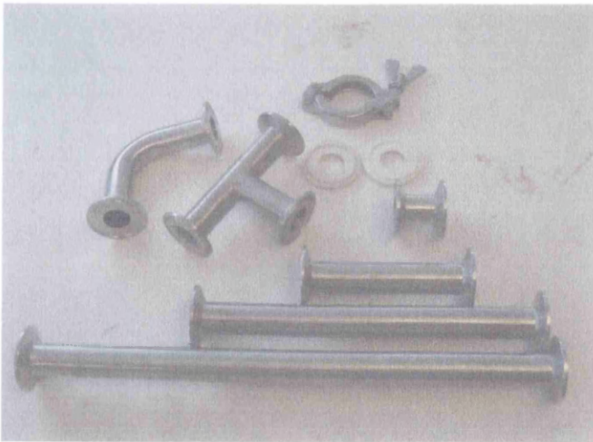
Fig.2.8. Photograph of all stainless steel SUS 316 clamps and pipes, and O-rings used to construct the MCR.
