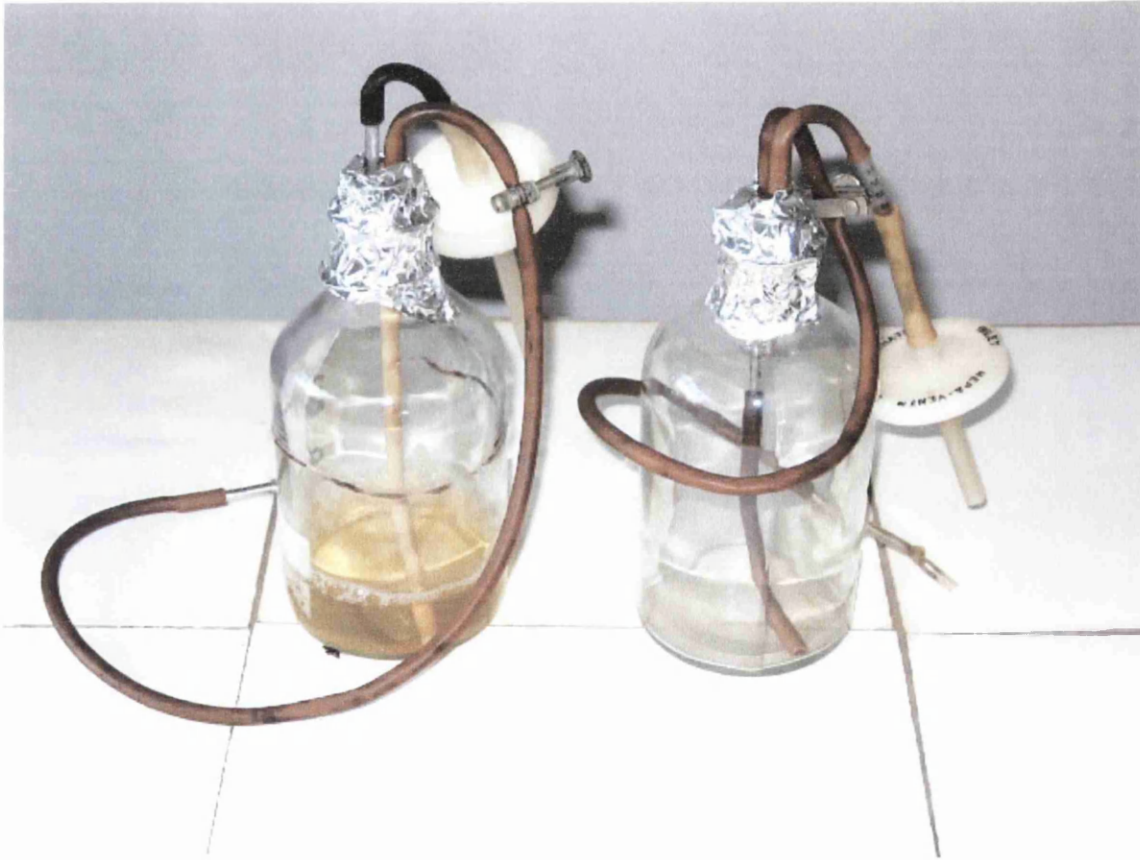
Fig.2.4. Starter culture bottles for inoculation into the STR. One bottle was used for the growth of the starter culture and for inoculation, and another was used for the feed of concentrated carbohydrate solution into STR just before inoculation. All tubes were made of rubber to prevent the culture system from exposing to the air. Long stainless steel tube reaches the bottom of the bottle and it was connected with inoculating line of STR. Short stainless steel tube was connected with high pressure nitrogen gas cylinder via the air filter and the manometer. Nitrogen gas from gas cylinder pressurized the starter culture bottle and pushed the culture liquid into STR through long tubing. All LAB were grown at this bottle for the starter culture, and both lines were blocked with clips to protect the culture from the contamination for cultivation.
