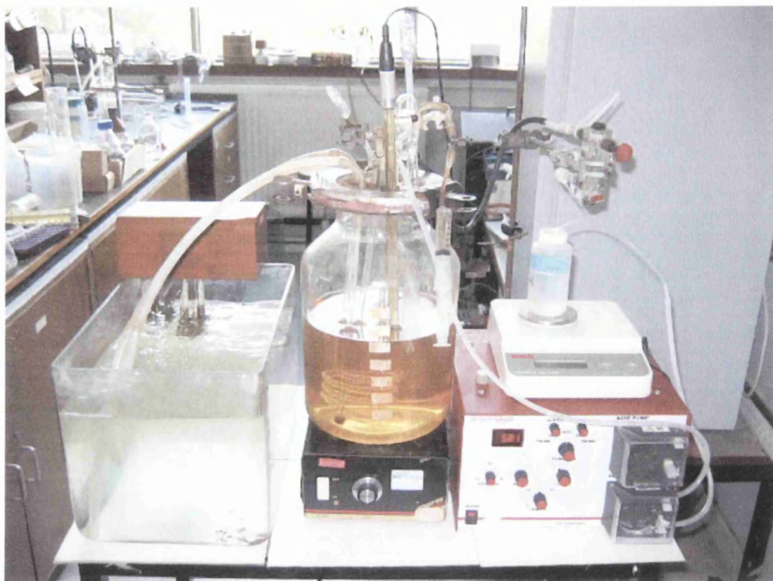
Fig.2.5. Photograph of the stirred tank reactor (STR) used to grow LAB. The bioreactor of total volume 5 L was agitated with magnetic bar on hotplate, and agitation speed was controlled by hotplate. Alkaline solution (5M NaOH) for pH control was reserved in the plastic bottle and its weight was measured with digital balance. Alkaline consumption rate was measured with reducing rate of the weight. Alkaline solution was fed with peristaltic pump controlled by pH controller. Temperature was controlled with the heat exchanger connected with the water bath. Another thermometer was fitted into the culture liquid was used to measure real temperature of the culture liquid.
