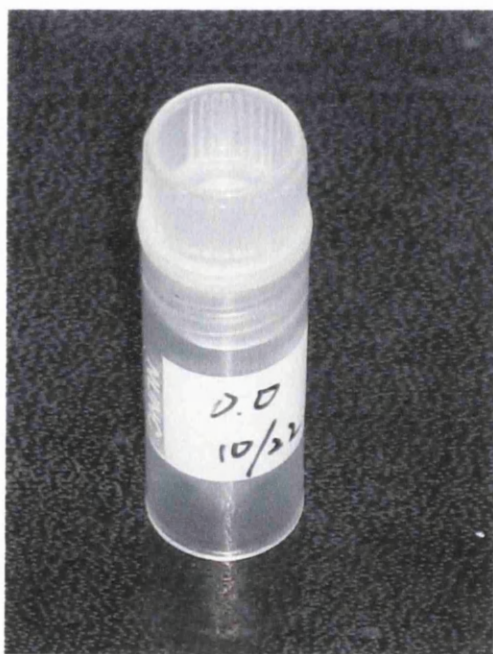
Fig.2.1. Photograph of the cryo-vial for preservation of the strains at - 70°C ultra-freezer.
