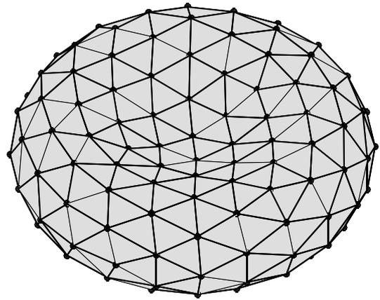
Fig 4. Full geometry of RBC membrane (problem domain) showing meshfree node distributions and triangular meshes as visualization aid.
