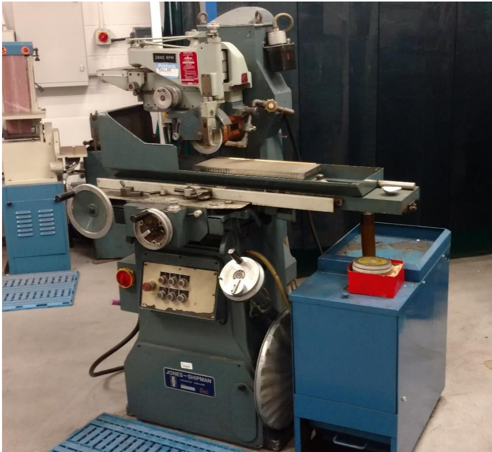
Figure 11 Jones Shipman 540 surface grinder fitted with magnetic bed chuck
