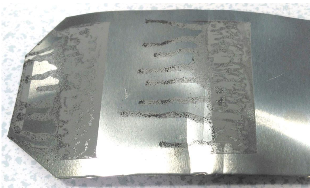
Figure 42 Electrode with thicker layer of active material – evidence of ink running during heating
