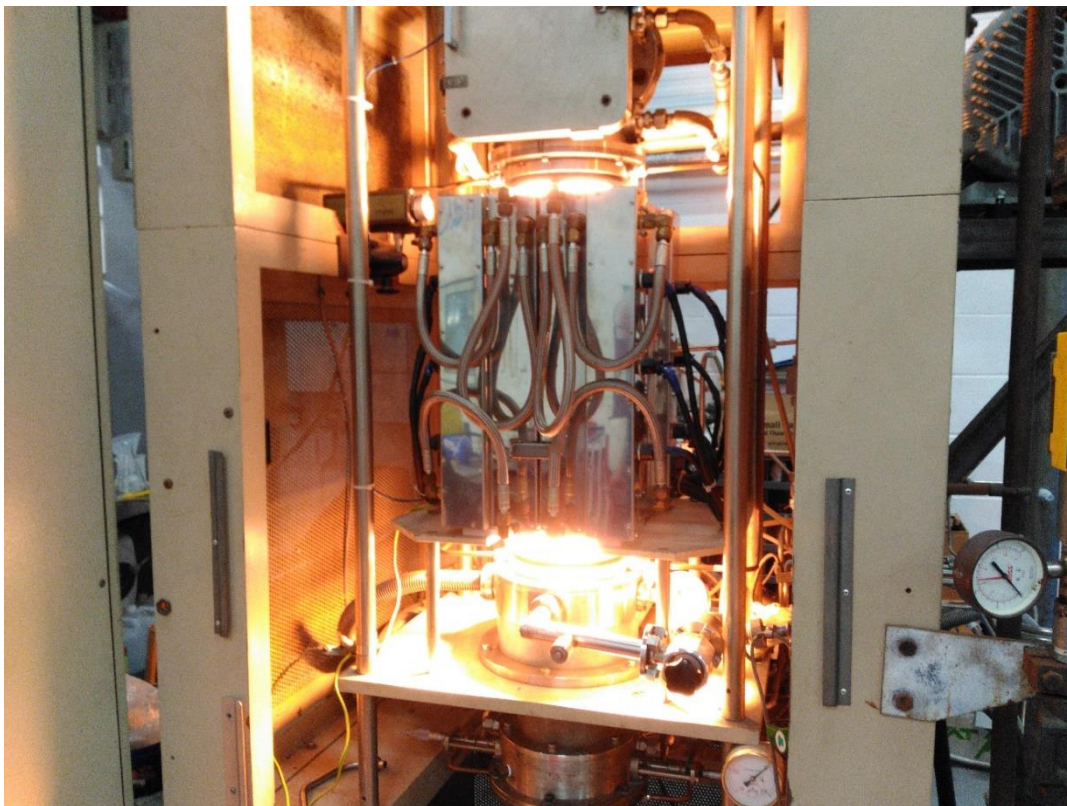
Figure 18 HDS Infrared Furnace during operation
