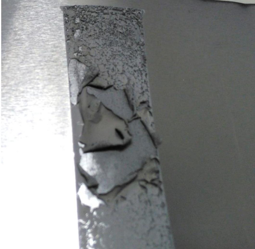
Figure 50 Sintered sample which had been cooled at a slower rate
