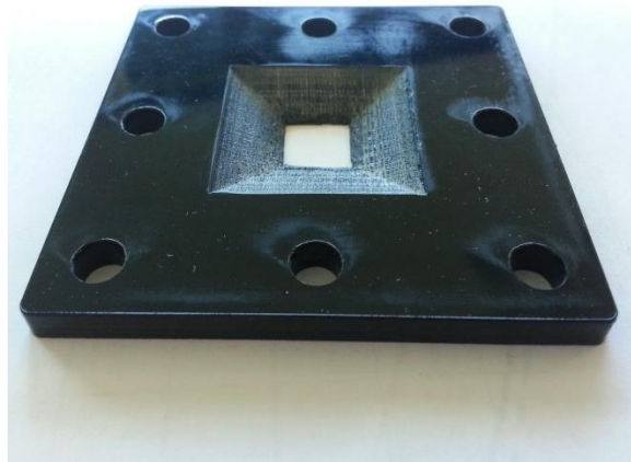
Figure 62 Chamfered profile cut using a laser cutter
