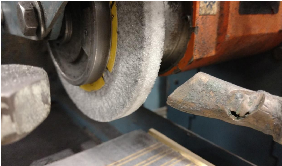
Figure 12 Flexovit grinding wheel above magnetic bed chuck
