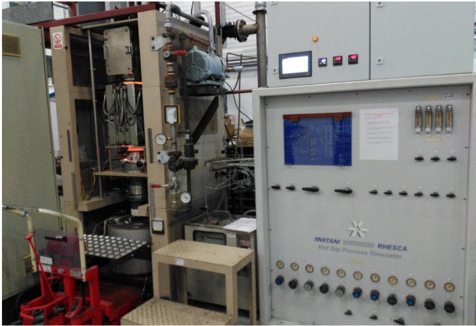
Figure 17 Iwatani Rhesca Hot Dip Process Simulator. Furnace - left. Control system - right
