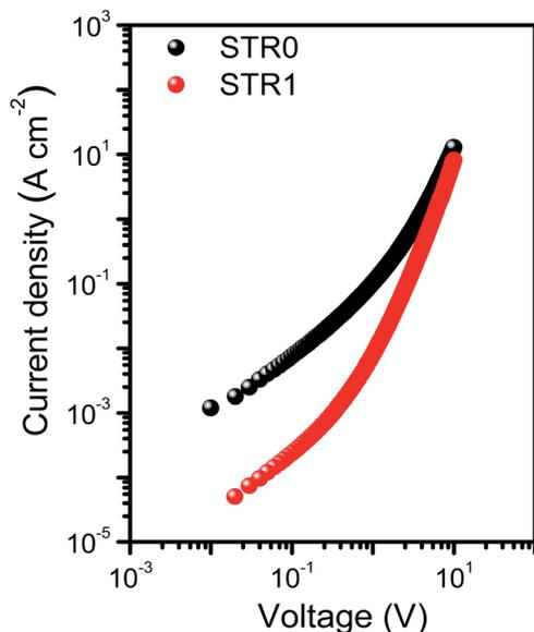
Fig. 4 Space charge limited current measurements with undoped STR1 and STR0 in the device configuration Si/SiO<sub>2</sub>/Au/PEDOT:PSS(AI 4083)/HTL/MoO<sub>3</sub>/Ag.
