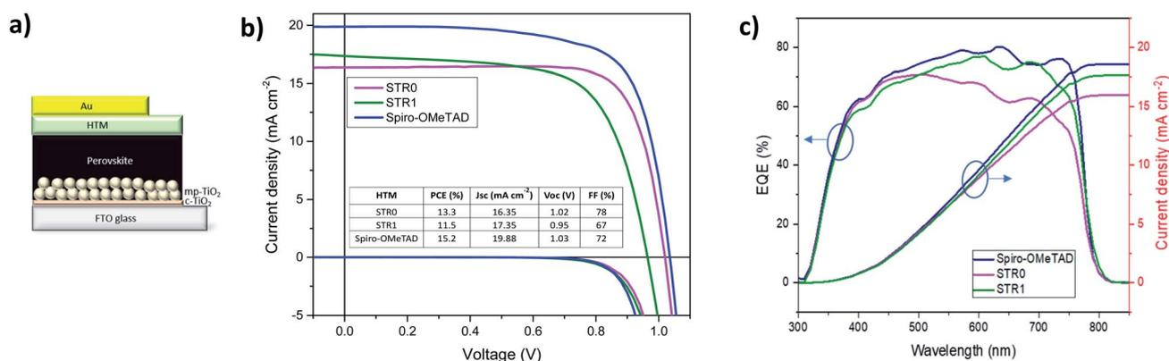
Fig. 5 (a) Device structure in the configuration FTO/bl-TiO<sub>2</sub>/mp-TiO<sub>2</sub>/CH<sub>3</sub>NH<sub>3</sub>PbI<sub>3</sub>/HTM/Au. (b)  $J$ - $V$  curves of the champion PSCs with STR1, STR0 and spiro-OMeTAD as HTMs measured after fabrication. (c) EQE spectra and integrated current density of devices with STR0, STR1 and spiro-OMeTAD.
