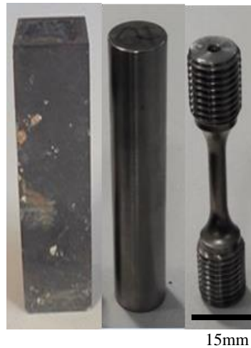
Figure 3.14: Examples of post heat treated blank, CNC machined cylinder and final fatigue test piece.
