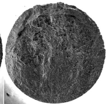
B18: 550MPa 828,200 cycles Surface
