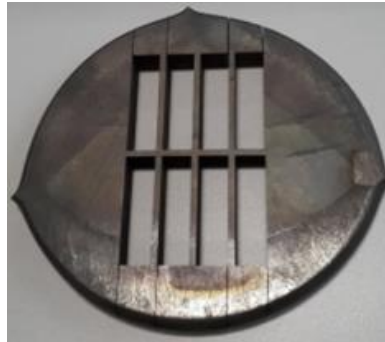
Figure 3.5: Extraction of specimen blanks from central regions of pancakes.
