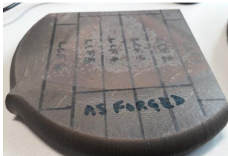
Figure 3.7: Third Ti-6-4 pancake from 8 inch diameter billet.
