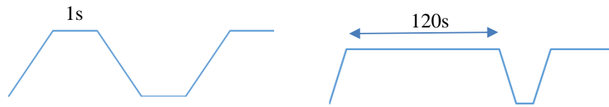
Figure 3.19: Schematic of (a) LCF and (b) Dwell waveform.
