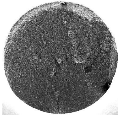
C01: 550 MPa 271,257 cycles Surface
