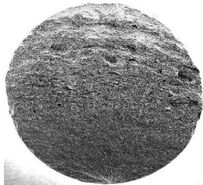
L06: 550MPa 92,880 cycles Surface
