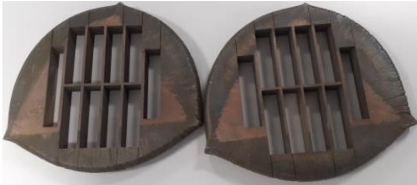
Figure 3.6: First two Ti-6-4 pancakes with blank extraction.
