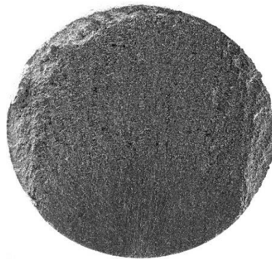
C02: 600MPa 65,994 cycles Surface
