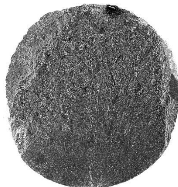
L07: 500MPa 131,698 cycles Surface
