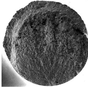
B10: 637.5MPa 73,400 cycles Surface
