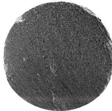
C05: 550MPa 1,879,081 cycles (1Hz)
