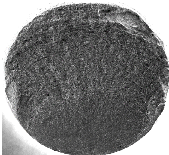
Figure 4.8: LCF fracture surface of a Ti-407 specimen from manufacturer 1.
