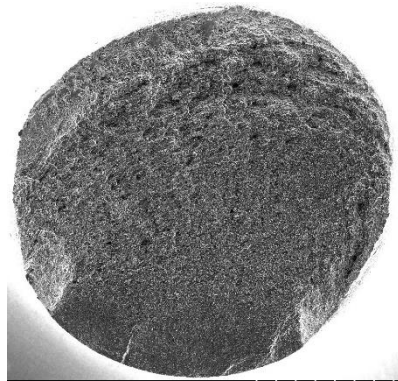
L04: 625MPa 13,176 cycles Surface
