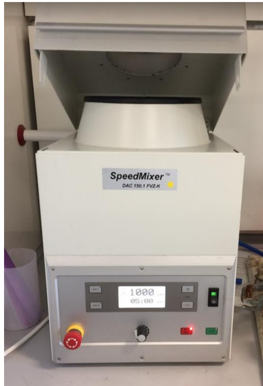
Fig. 7 - 1: Image of a Speed mixer DAC150.1 FVZ.K employed during pigmented model fluids preparations
