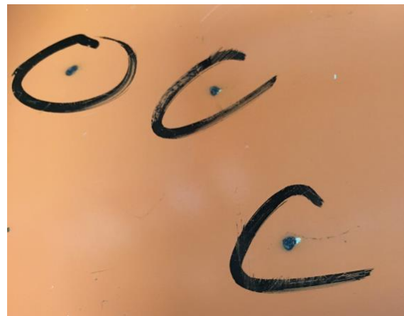
(b) Coating debris defect
