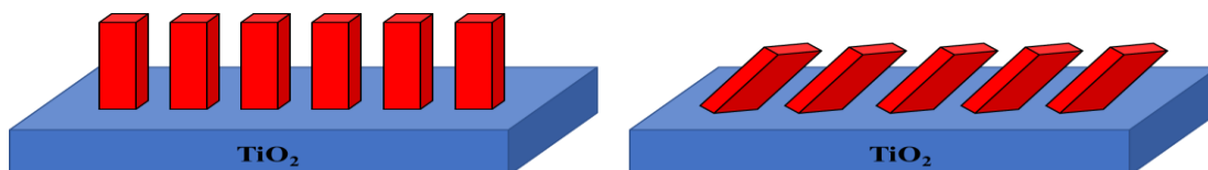
Figure 1.22 – Dye orientation on \text{TiO}_2 . Dyes perpendicular to \text{TiO}_2 (left). Dyes at a 45^\circ angle to \text{TiO}_2 . Dyes in red, \text{TiO}_2 in blue.
