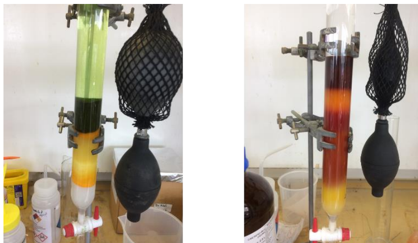
Figure 3.5 - (left) column chromatography of C(CH_3)_2 -containing dye (7) showing green due to the combination of yellow/red half-squaraine along with a blue full-squaraine impurity and (right) the synthesis of sulphur-containing dye (6), which only shows the red/yellow colour of half-squaraine.
