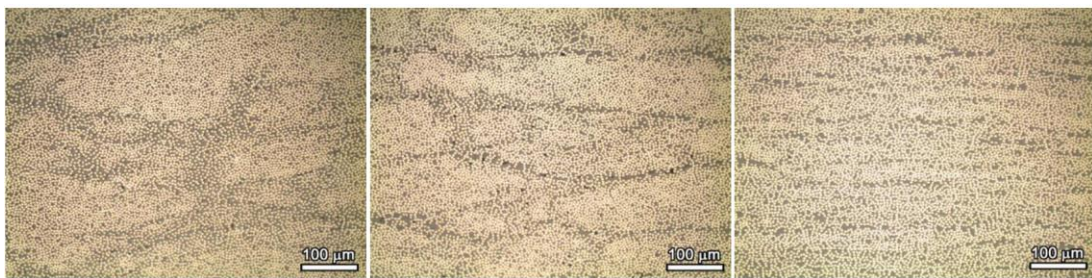
Figure 2.16 Micrographs of unidirectional laminates made from various thickness prepregs (left 300 g/m 2 , middle 150 g/m 2 , right 50 g/m 2 ) [74] 4
