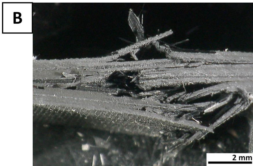
Figure 4.17 QI unnotched compression failure modes: a) 50 g/m 2 , b) 150 g/m 2
